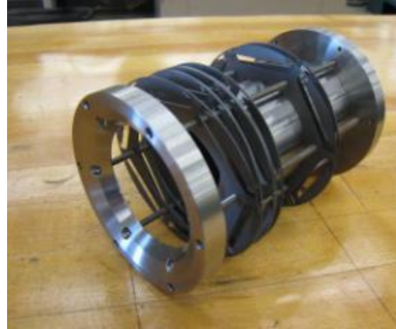
Figure 4-160: Shaft adapter, opposite lead end clamp ring, and several laminations.
