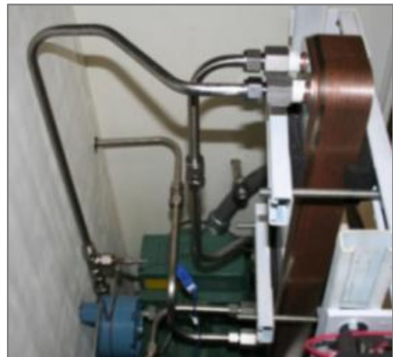
Figure 4-113: Side view of brazed plate internal heat exchanger
