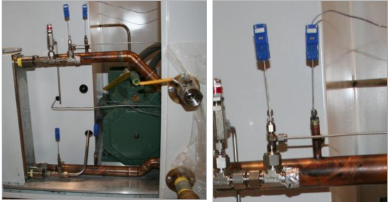
Figure 3-21: Pressure and Temperature Measurement on the Water and Refrigerant Side of the Gas Cooler
