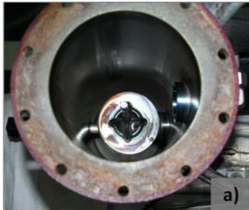
Figure 4-134: Opened phase separator without splash plate
