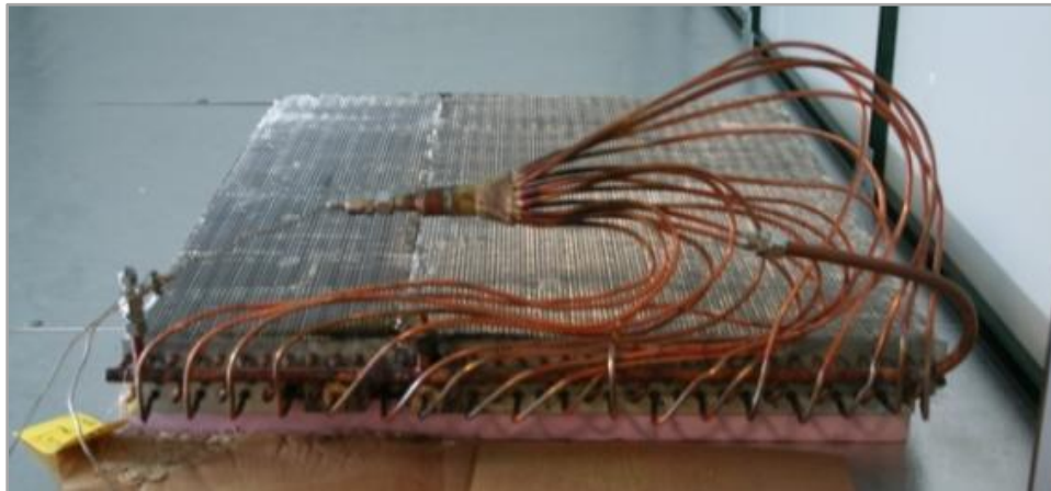
Figure 4-51: Assembled enhanced evaporator
