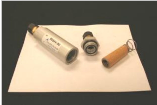
Figure 4-54: Inline filter before system flushing
