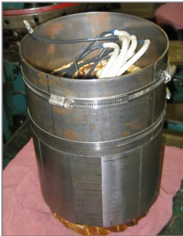
Figure 4-193: Pressing ring installed on stator
