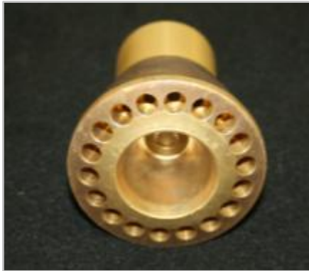
Figure 4-50: Distributor for enhanced evaporator
