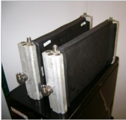
Figure 4-8: Internal heat exchanger with insulation (left) and mounted piping (right)
