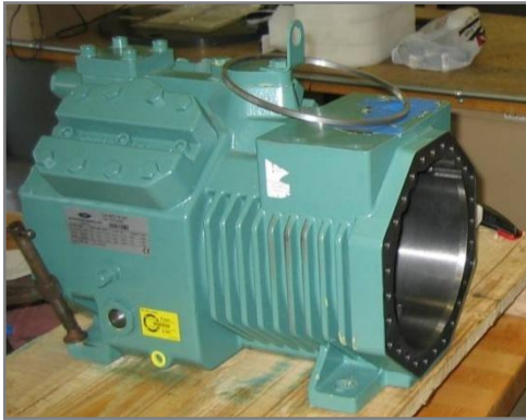
Figure 4-191: Compressor, 36 slot 6 pole stator and spacing ring readied for insertion
