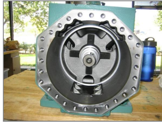
Figure 4-192: Spacing ring installed in compressor bore
