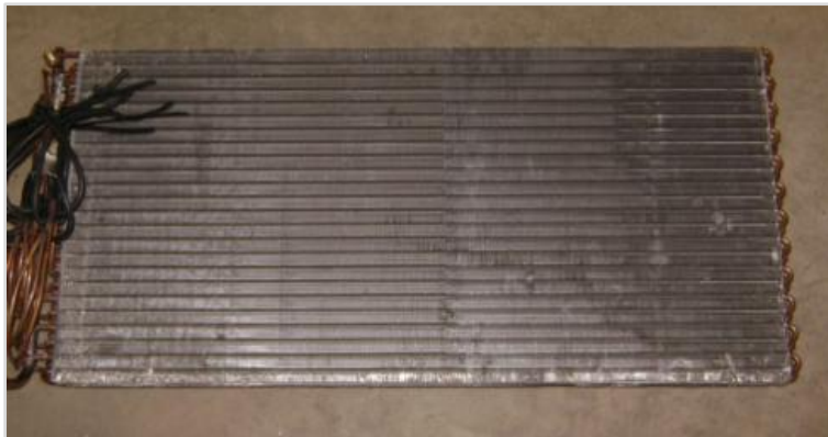
Figure 3-2: Evaporator for Baseline R744 Heat Pump Water Heater
