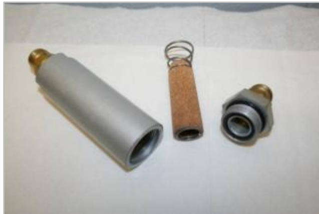
Figure 4-55: Inline filter after system flushing
