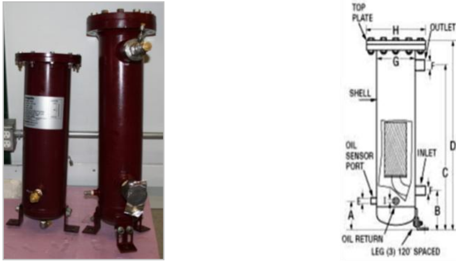
Figure 4-114: Comparison of smaller phase separator from previous investigations and new larger component
