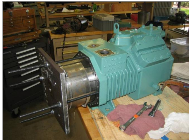
Figure 4-194: Partially pressed in 36 slot 6 pole stator
