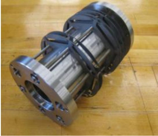
Figure 4-160: Shaft adapter, opposite lead end clamp ring, and several laminations.
