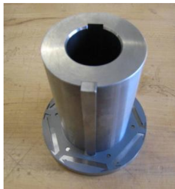
Figure 4-161: Rotor shaft adapter with a single lamination
