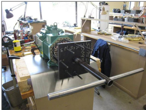
Figure 4-189: Back bolts and plate with large custom made nut driver.
