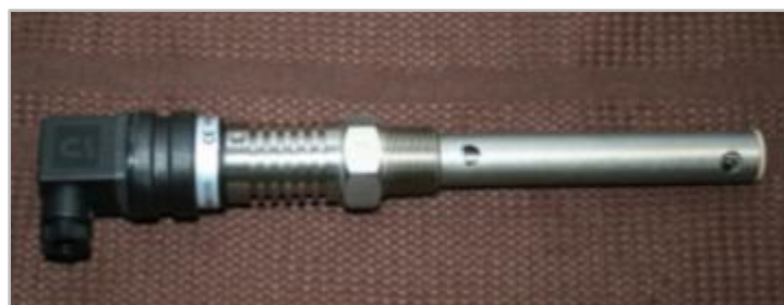
Figure 4-99: CO 2 liquid level sensor
