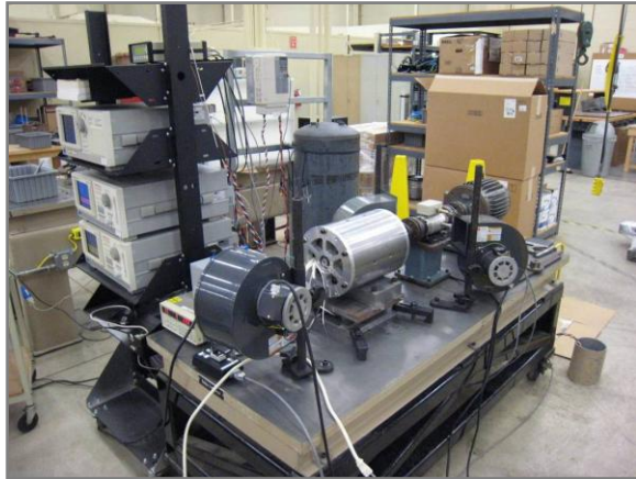
Figure 4-167: Light load dynamometer set up
