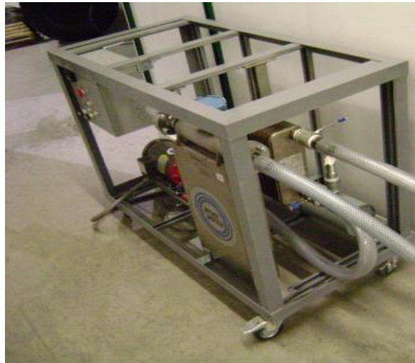
Figure 2-7: Water/Glycol Measurement Cart
