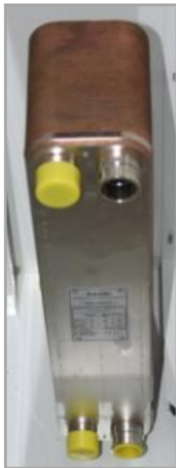
Figure 3-14: R744 Brazed Plate Gas Cooler
