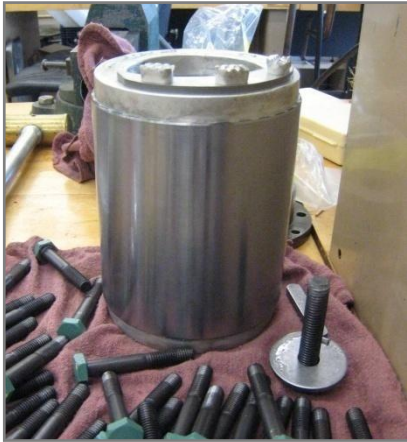
Figure 4-187: Stock induction machine rotor and holding nut.
