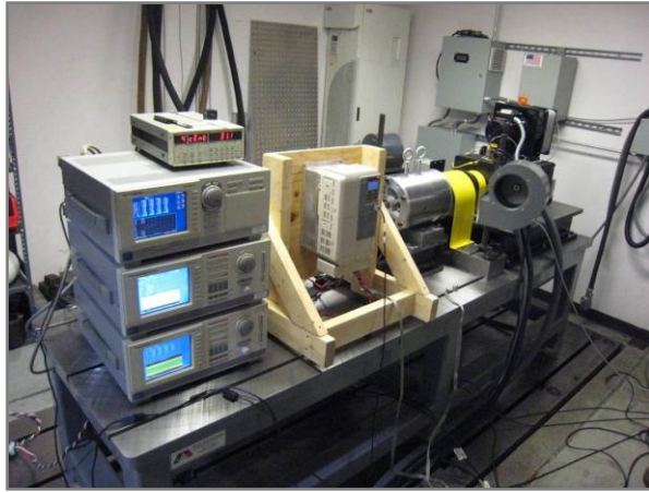
Figure 4-174: Full load dynamometer with data acquisition equipment
