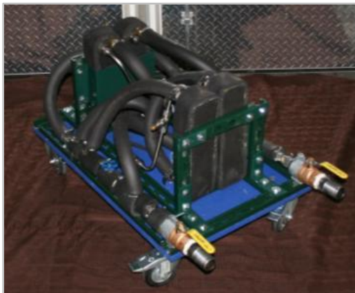
Figure 4-77: Multiple gas cooler cart
