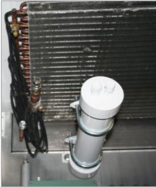
Figure 3-18: Accumulator and Evaporator with its Refrigerant Distributor
