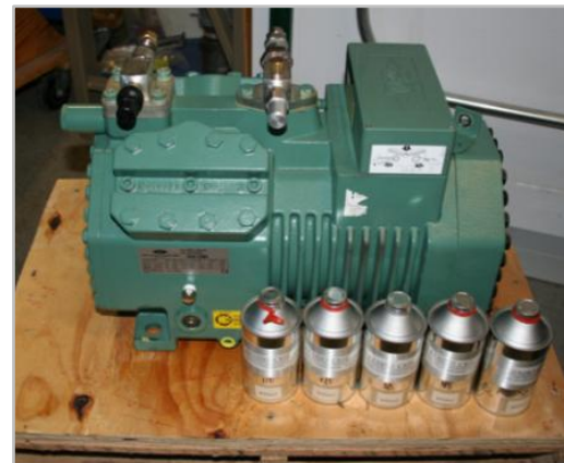
Figure 4-199: Compressor with suction and discharge port after addition of oil
