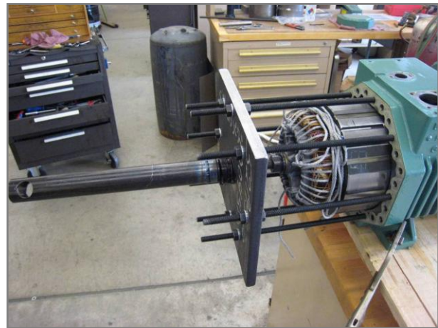
Figure 4-190: Partially extracted induction machine stator
