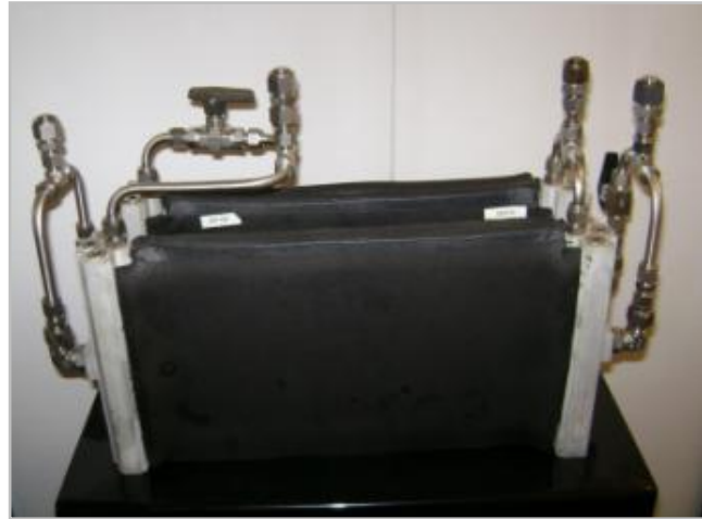
Figure 4-8: Internal heat exchanger with insulation (left) and mounted piping (right)
