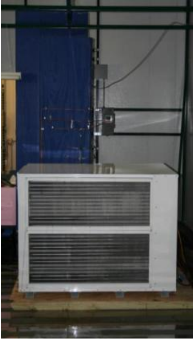
Figure 2-4: Evaporator Wind Tunnel Connected to Baseline R134a System
