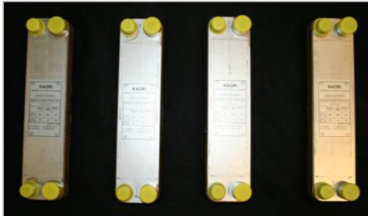
Figure 4-75: Brazed plate heat exchangers for gas cooler optimization
