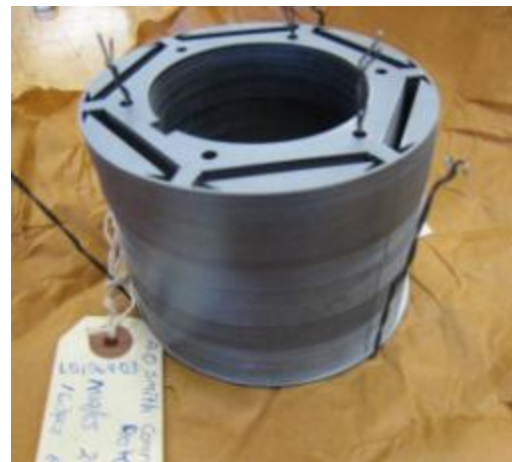
Figure 4-158: Laser cut common rotor laminations.
