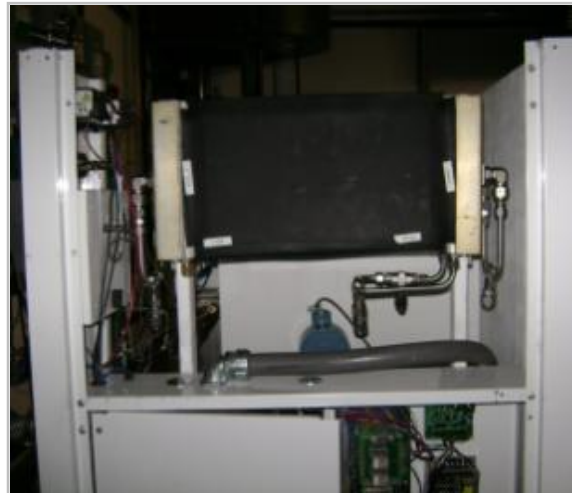
Figure 4-10: HPWH with installed IHX
