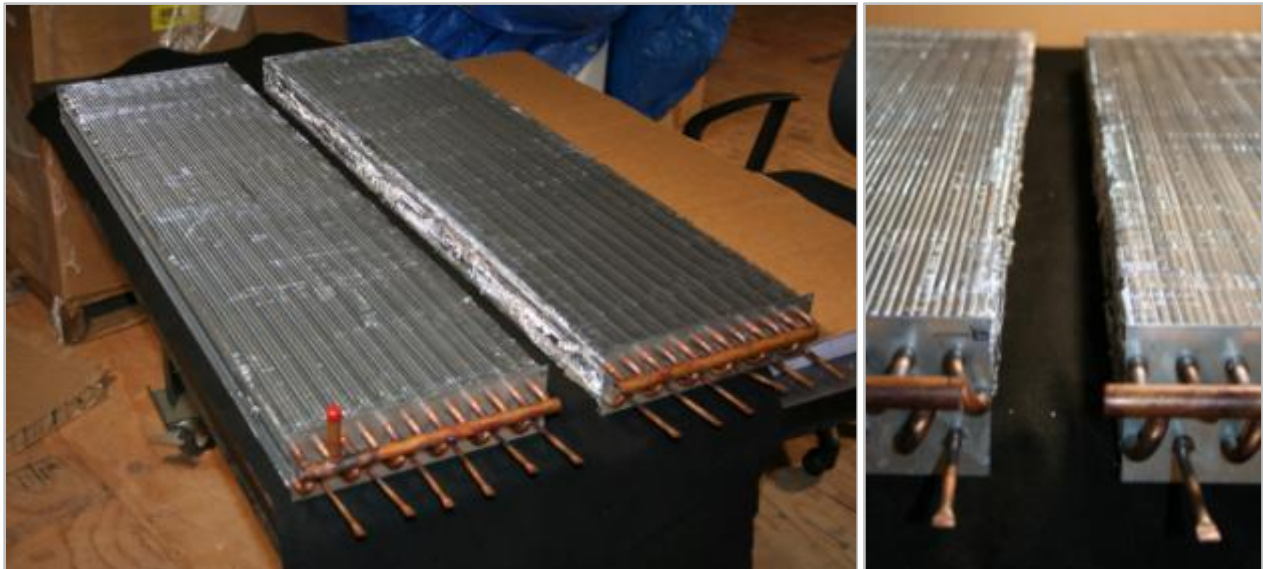
Figure 4-49: Cut evaporator halves and detailed view of section plane
