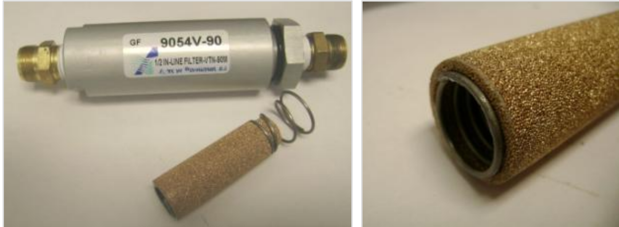
Figure 4-16: Inline filter after 3h system run
