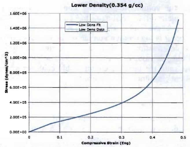
Figure 4. Uniaxial strain compression data and fits to PDMS foam with a density of 0.354 g/cc, an approximate initial porosity of 0.68.
