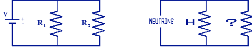
Figure 1: Resistors in parallel compete for electric current (left) just as multiple neutron-capturing elements in solution compete for neutrons (right).
