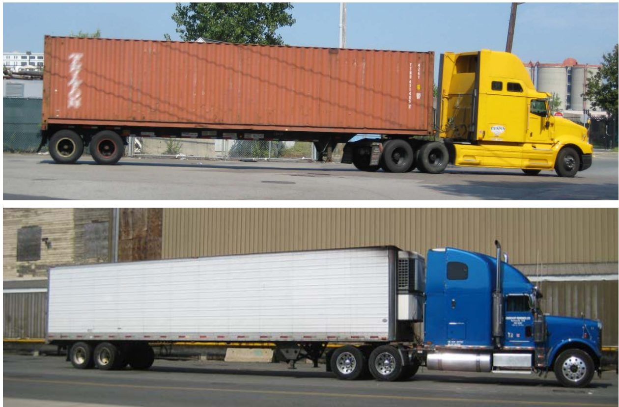
Figure 4.4. Truck hauling intermodal container on a trailer chassis (top), and truck hauling conventional dry van (bottom)
