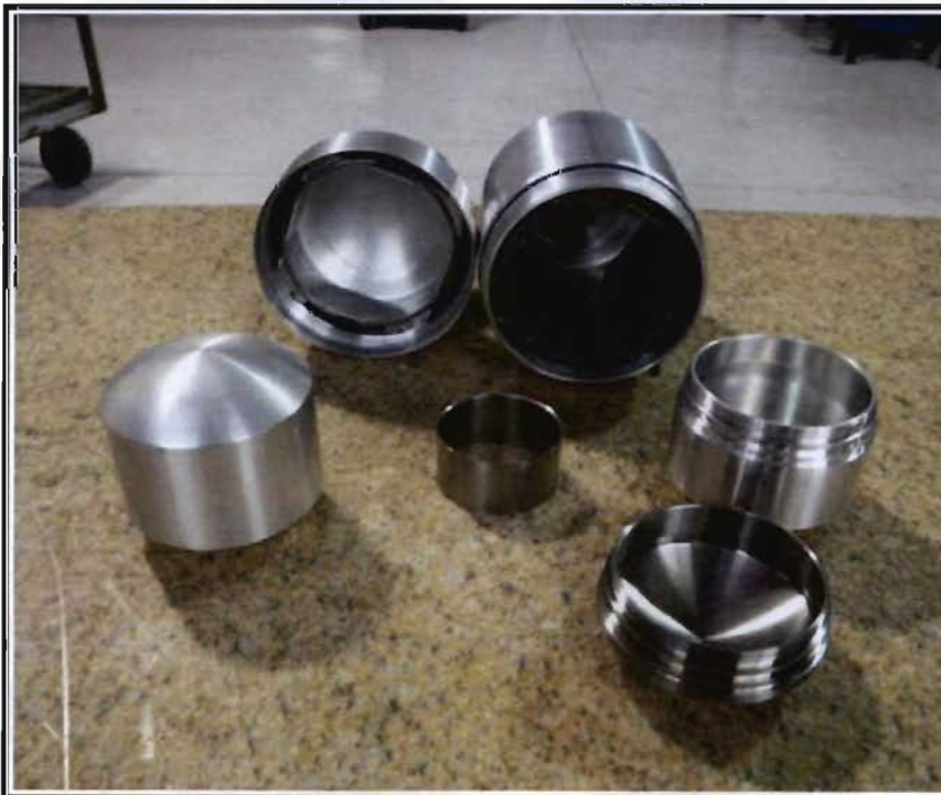
Figure 9: Sample Containers Size 2 (SC-2) and T-Ampoule with Cradle Assembly Installed
