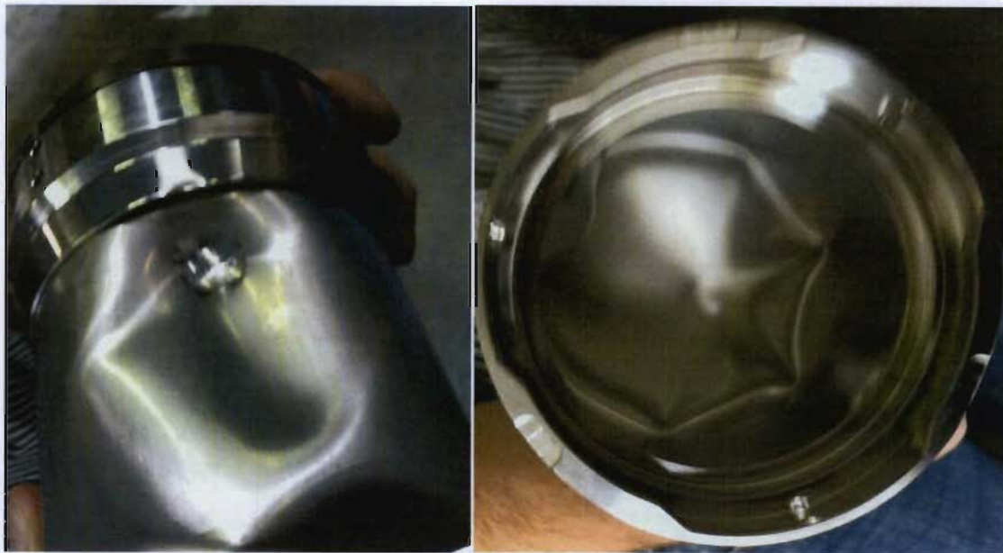
Figure 4. Damage Caused by Penetration Bar (Left: near weld, Right: bottom)
