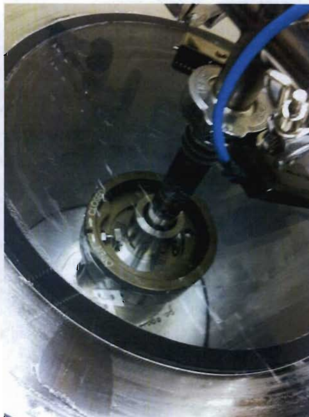
Figure 5. Helium Leak Testing of the Container After Penetration Tests
