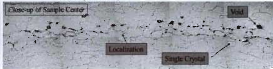
"Void sheets" are forming along grain boundaries in sample
