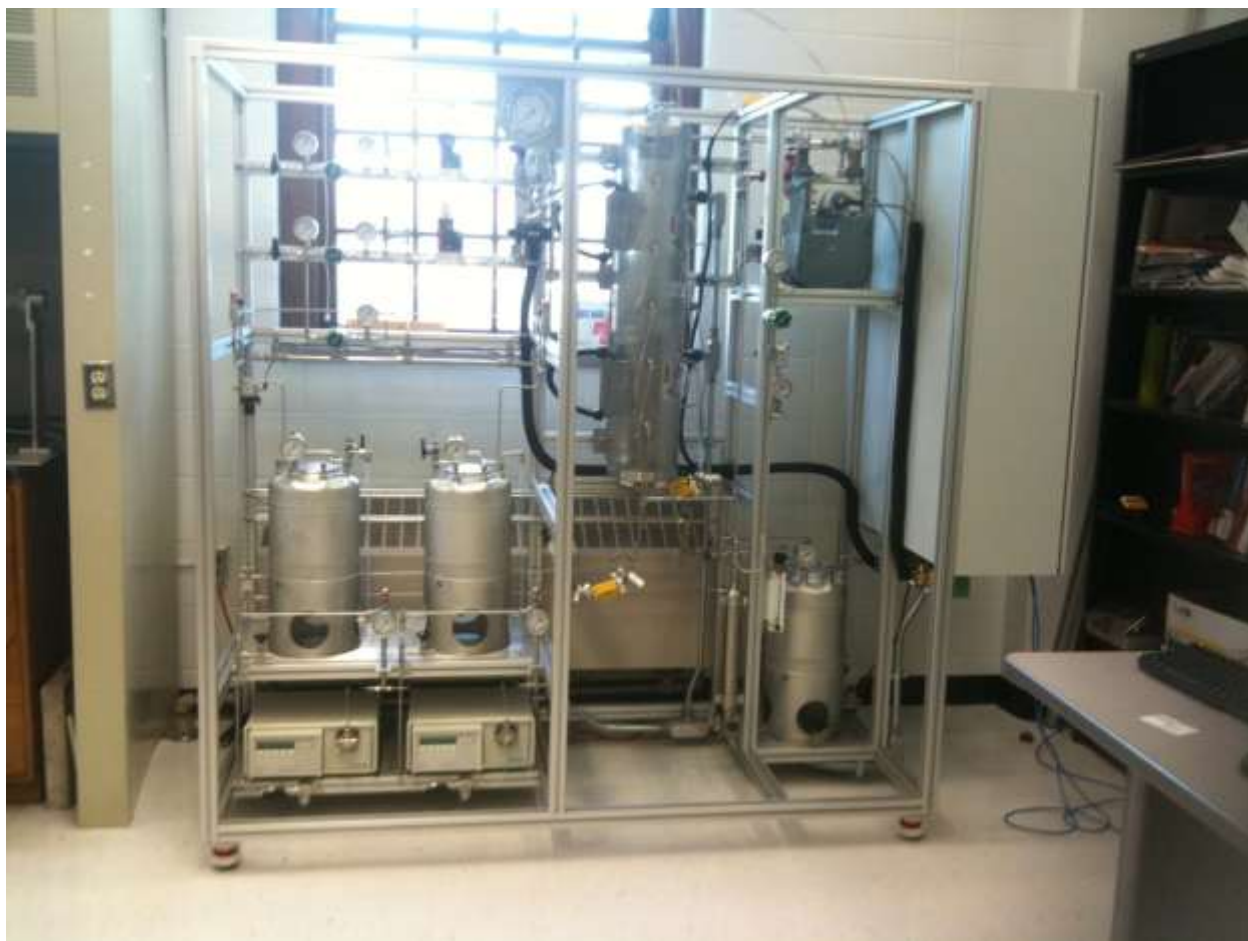
Figure 1. Reactor Unit for heterogeneous catalytic reactions: Designed, fabricated and commissioned at Conn Center.
