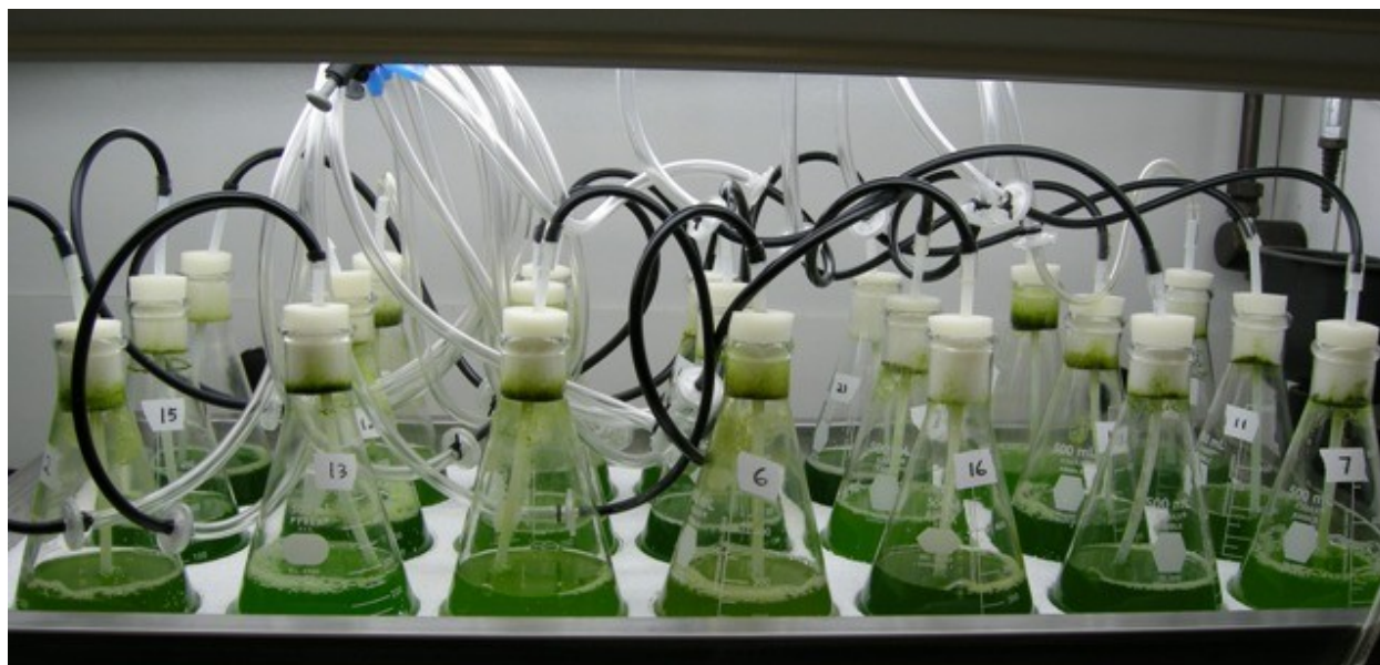
Figure 5. Algae culture system used in a simulated flue gas experiment with 21 flasks on a shaker table.
