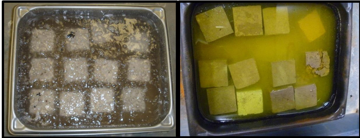
Figure 3: Concrete Cube Specimens during Thermal Cycling Tests
