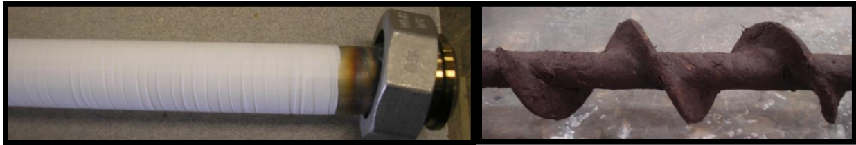
Figure 7: Plain Tube Heat Exchanger with Teflon Tape Interface (Left) and Auger-Fin Heat Exchanger with Deacon Paste Interface (Right)
