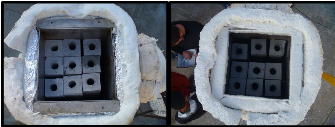
Figure 12: Concrete Beams in Thermocline Tank before (Left) and After (Right) Preliminary Testing
