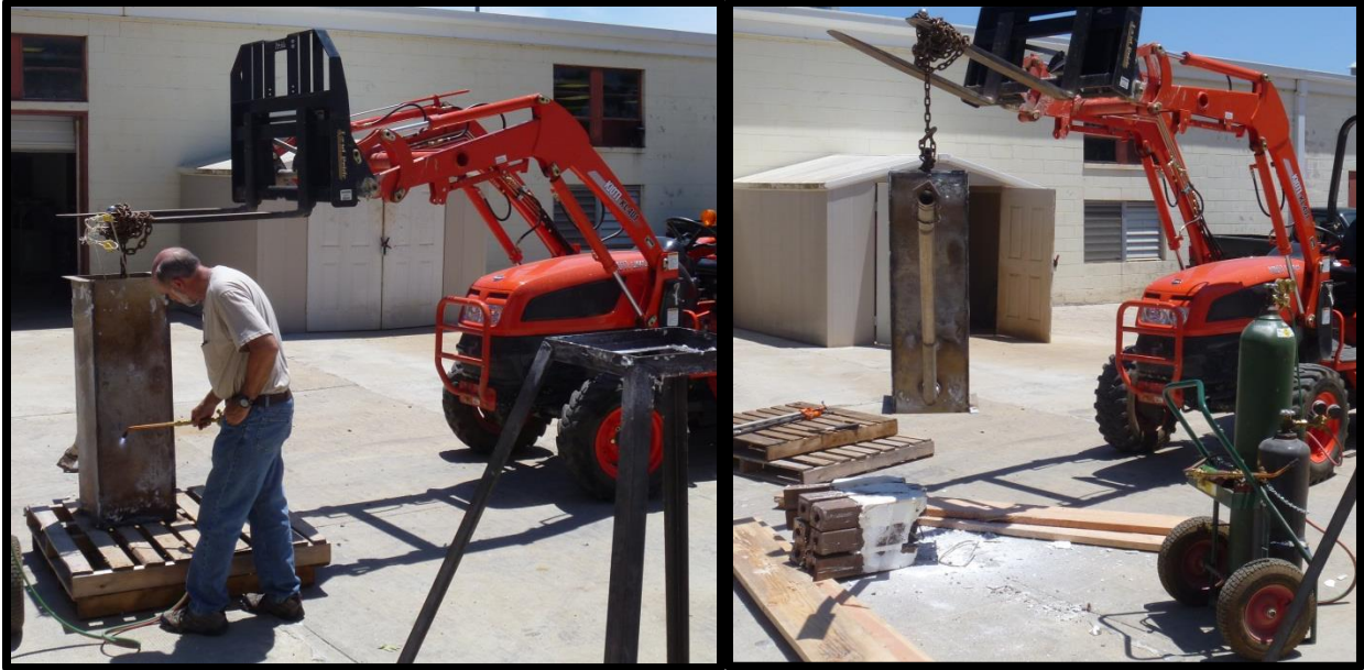
Figure 14: Heating Frozen Thermocline Test Chamber (Left) and Cleared Thermocline Chamber with Concrete/Salt Blockage on the Ground (Right)
