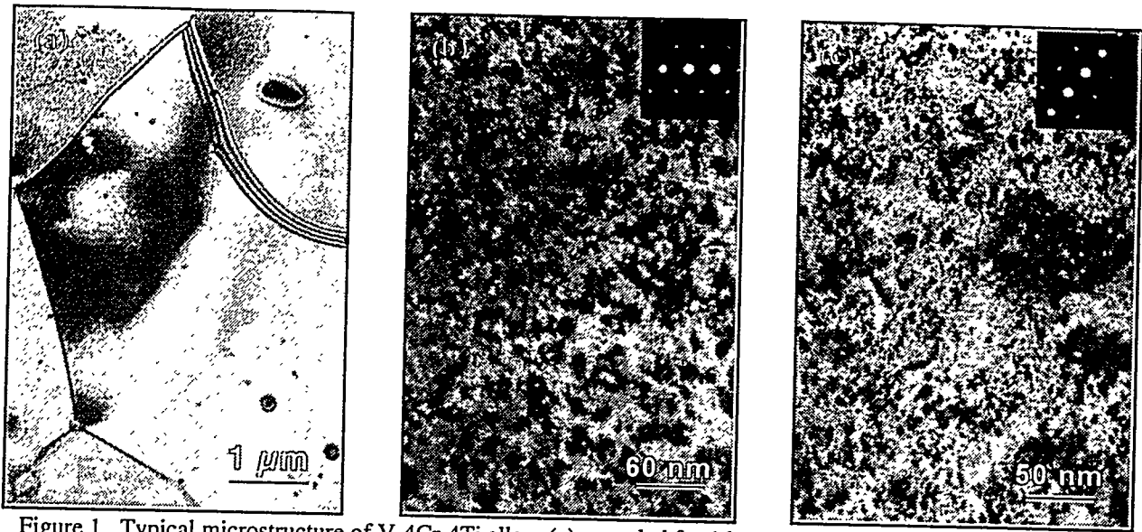
Figure 1. Typical microstructure of V-4Cr-4Ti alloy: (a) annealed for 1 hr at 1050°C in UHV furnace, (b) ion irradiated to 5 dpa at 350°C with 4.5 MeV Ni 2+ , and (c) irradiated to 4 dpa at 390°C in the X530 experiment.
