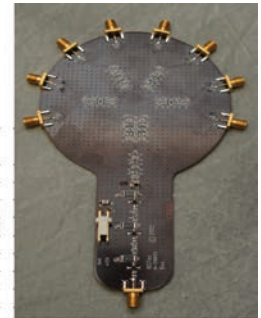
Figure 6. The new clocking circuit has 3.248 ps of random jitter. This is a significant improvement over the 300 ps jitter specification on the PLLs in the FPGA.
