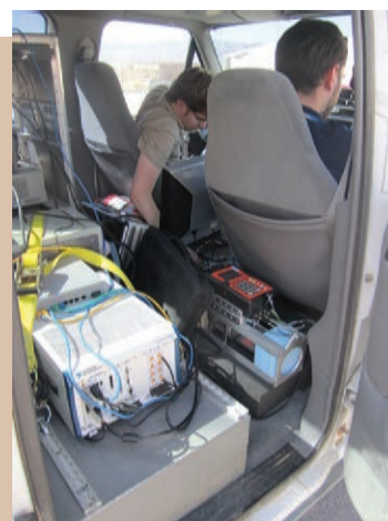
Operational testing was conducted by placing the system in a vehicle and equipping it with several detectors
