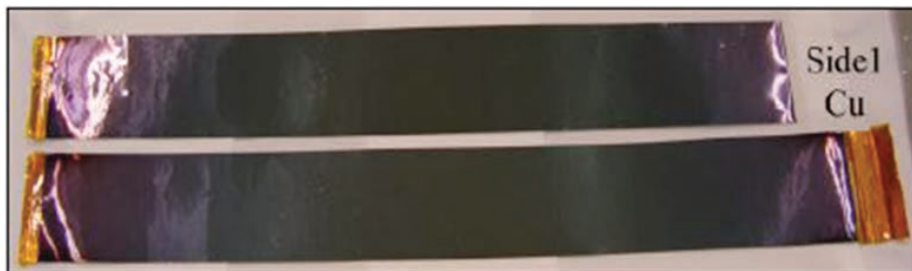
Figure 3. The copper foils coated with ^{10}\text{B}
