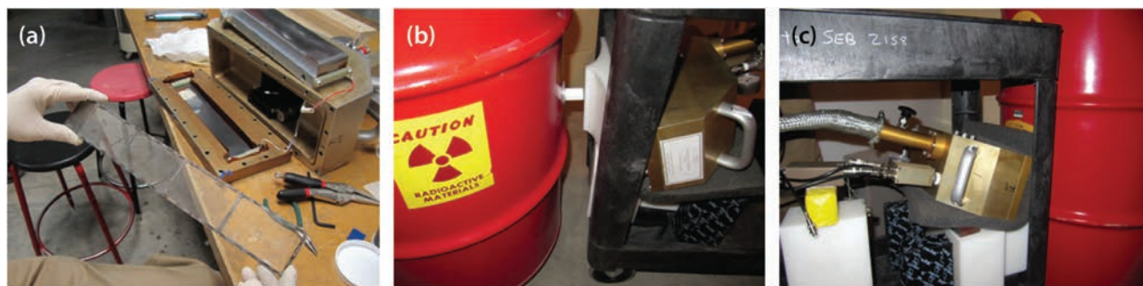
Figure 7. (a) The box chamber is seen with interior exposed. The mesh was installed inside a stainless steel frame. (b) The detector was exposed to the source through a 25.4 mm diameter porthole. (c) The detector was placed on foam, and moderator blocks were stacked nearby to thermalize the fast neutrons from the PuBe source.
