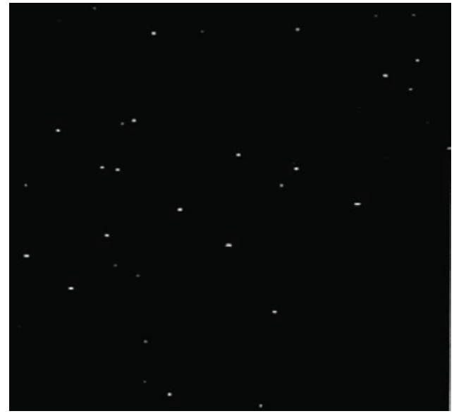
Figure 3. Unrecoverable specks of CCD image sensor (DT neutron fluence: 8 \times 10^7 neutrons/cm 2 )
