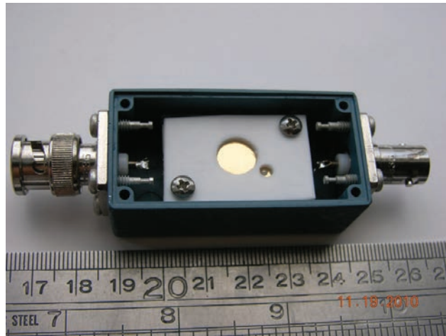
Figure 2. CZT mounted in a Pomona shielded box
