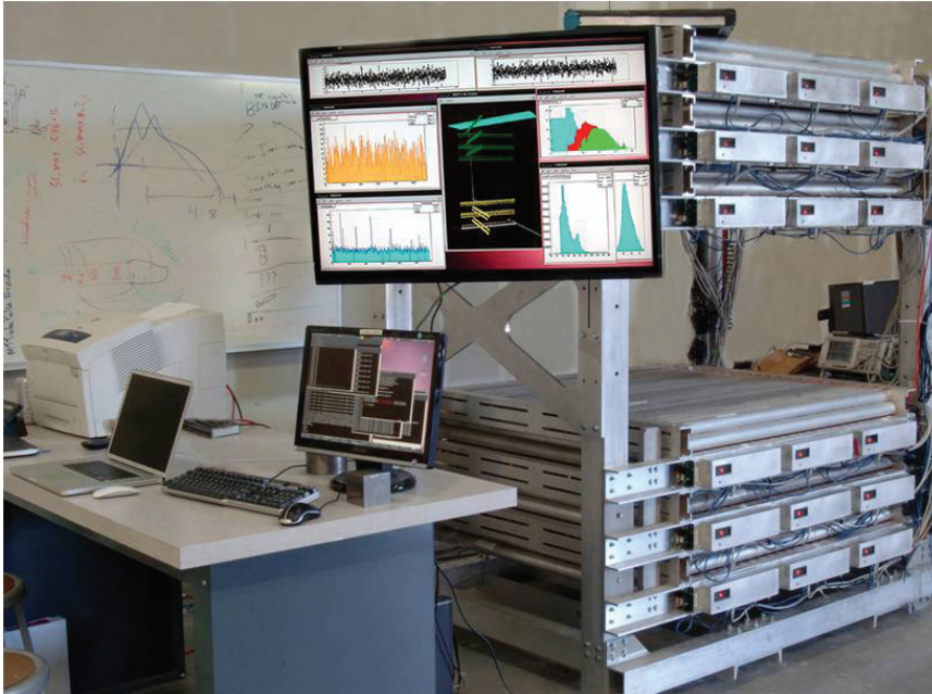
Figure 2. The mini muon tracker (MMT) was built at Los Alamos for muon tomography applications. There are 24 planes of 4-foot long drift tubes to track muons in x and y directions.
