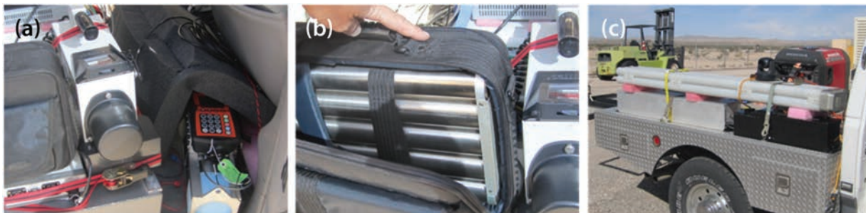
Figure 8. (a) Mechanically cooled and LN 2 -cooled HPGe detectors, (b) 13-inch 3 He array, and (c) 36-inch 3 He array configured for final operational testing
