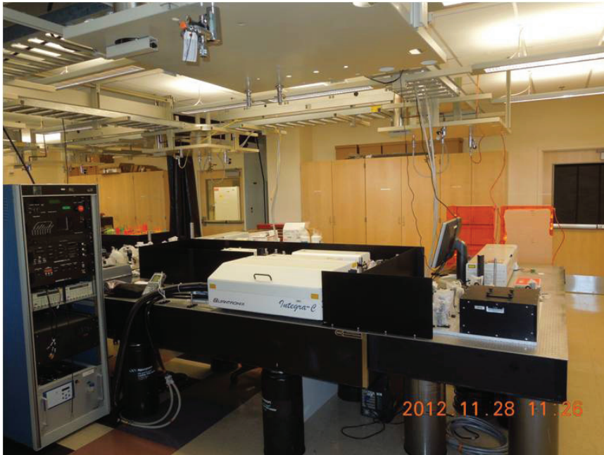
Figure 1. The UNLV laboratory for AlGaN device characterization. TOPAS, a femtosecond widely tunable optical parametric amplifier, is installed in the lab.
