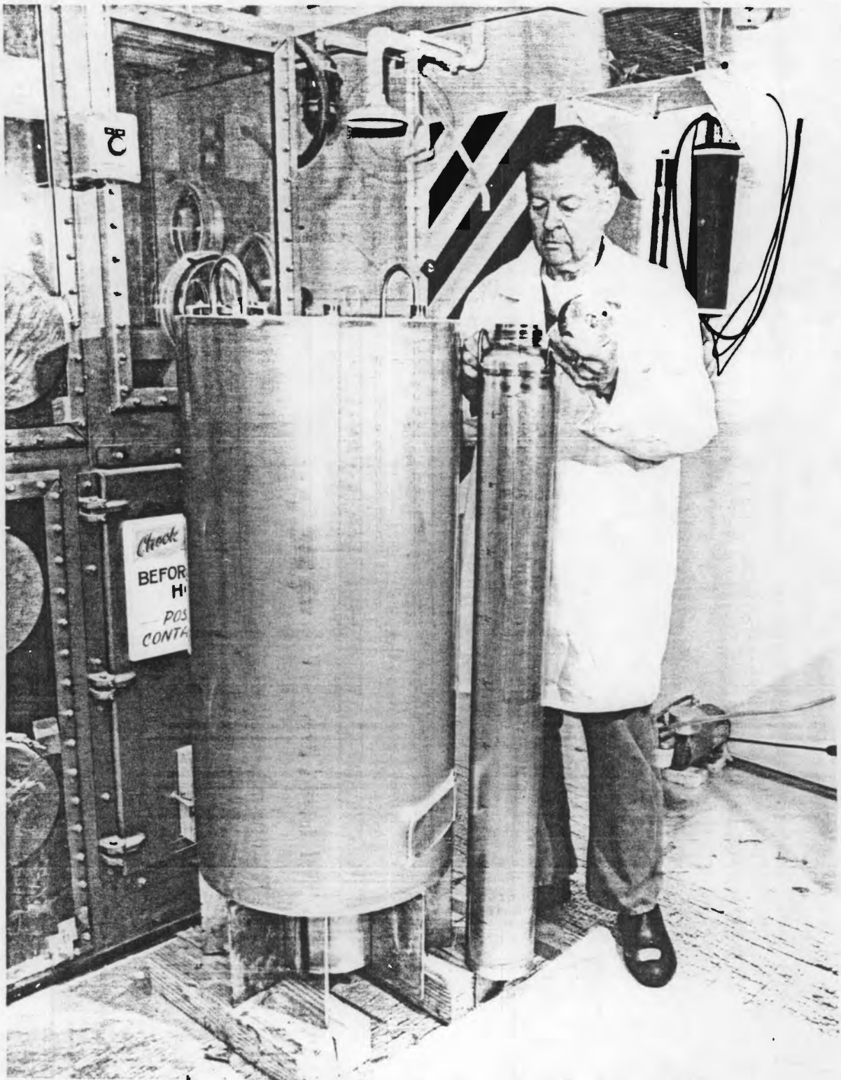
FIGURE 2.7 Photograph Showing Annular Tank and Bottle
