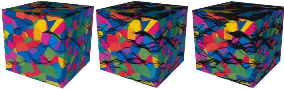
The figures show progress of phase transformation in iron under high rate loading conditions. Dark regions have transformed from Alpha to Epsilon phase.
