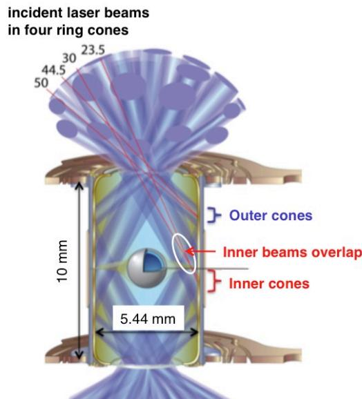
The figure shows a schematic of a NIF ignition target showing the inner and outer beam cones and the VPIC simulation region where inner beams overlap.
