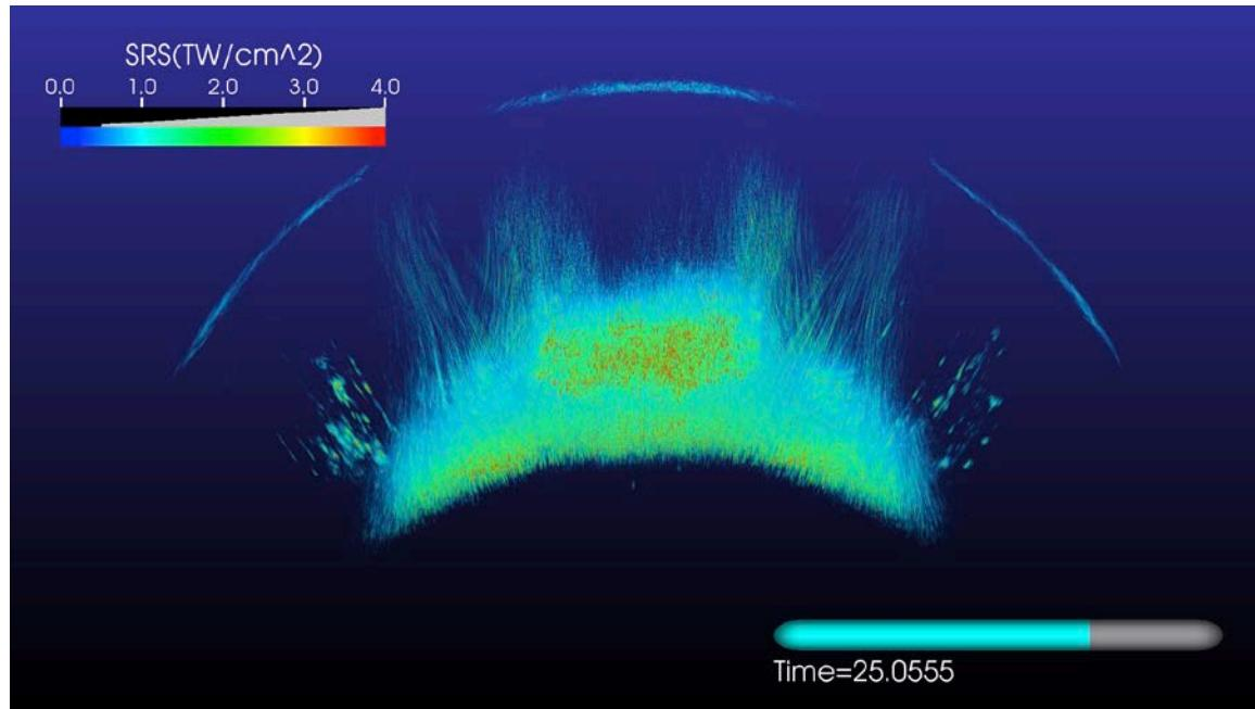
This figure shows a volume visualization of the laser light backscattered by Stimulated Raman Scattering (SRS). The SRS occurs in bursts and is shown near the end of a burst when the scattered light comes mostly from the region where the quads overlap (the arc of light at the bottom).
