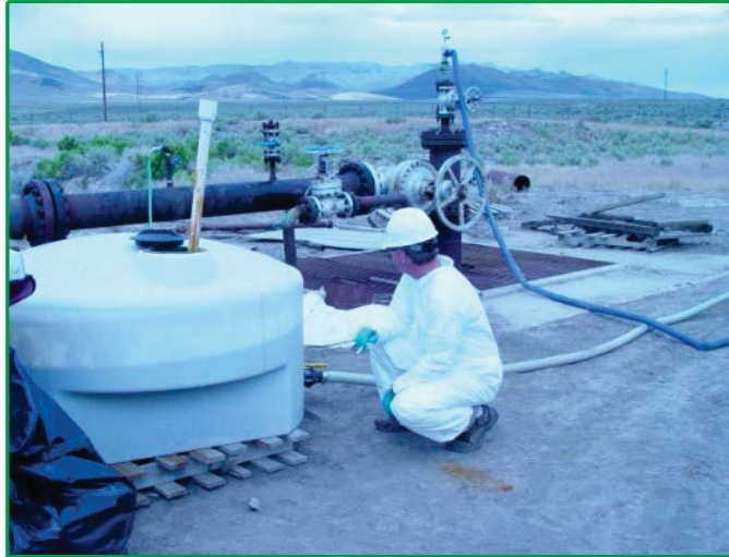
Figure 31. Injection of naphthalene 2,6-disulfonic acid sodium salt and acetamide at well RRG-5 on July 21, 2010.
