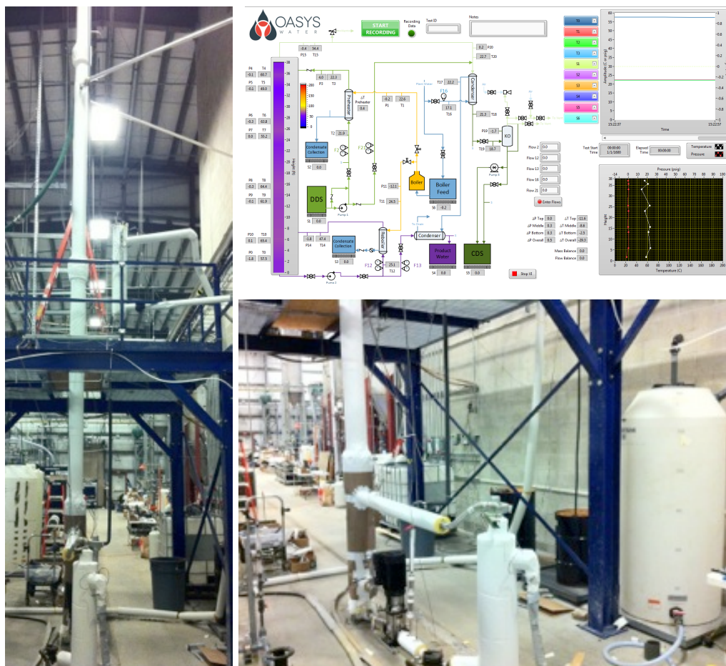
Figure 4: Photographs of pilot stripper and absorber system and screen capture of associated human machine interface of the data acquisition and control system.
