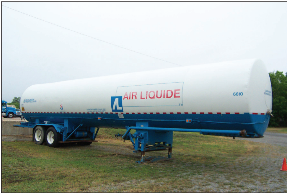
Figure 52. Air Liquide 54.4-tonne (60-ton) portable CO 2 storage tank. Photograph was taken by Mike Griffith for Air Liquide.
