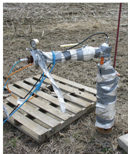
Figure 16. Design of M-1 wellhead (at left) and photo of M-1 (at right). This design is representative of all the monitoring wells. Insulation and heat tape in photograph are to protect the wellhead during the winter months.
