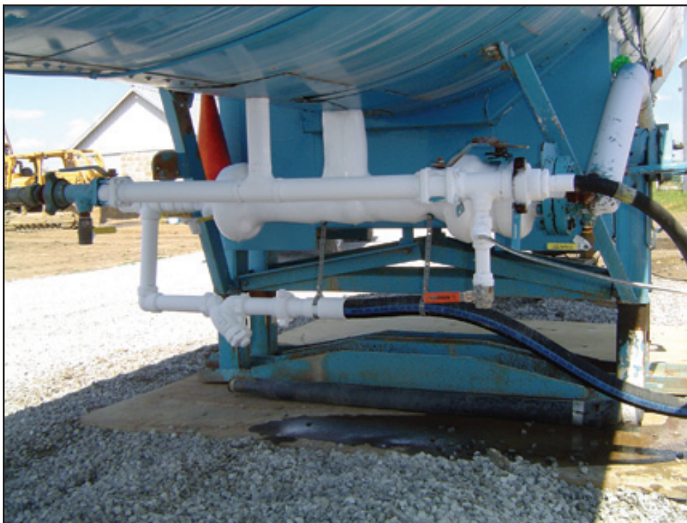
Figure 53. The outlet (bottom) and inlet (top) lines underneath the portable CO 2 storage tank. The black flexible hose with blue stripe runs to the booster pump (liquid CO 2 supply hose) and the solid black hose is the liquid and vapor return from the pump skid. Photograph was taken by Ray McKaskle for Trimeric Corporation.
