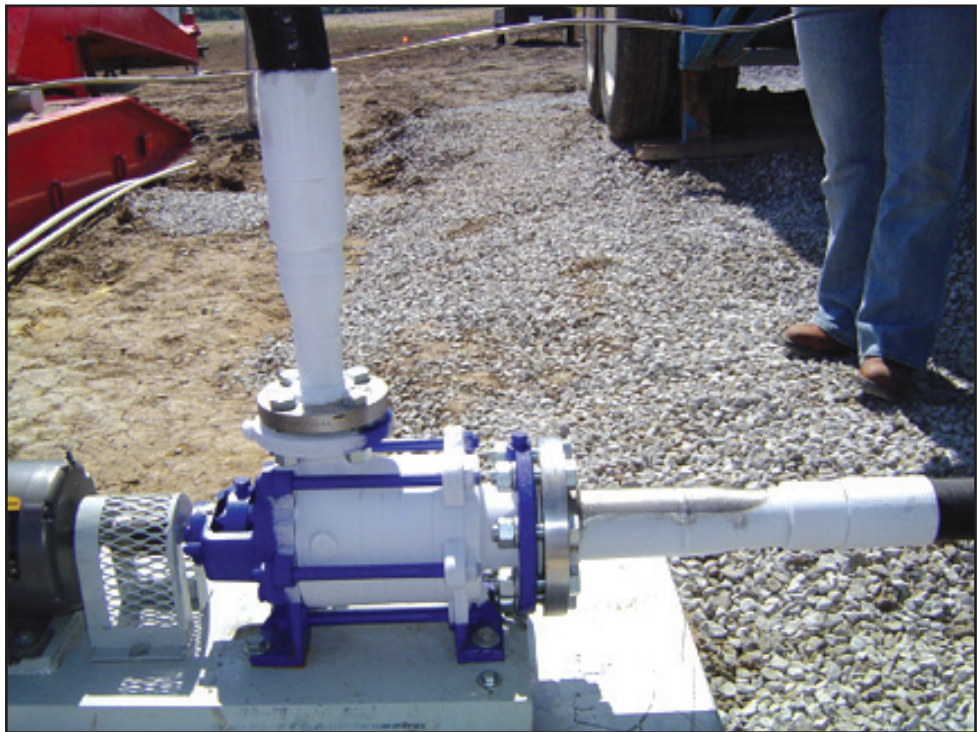
Figure 54. Booster pump model SRZS 221, horizontally mounted side channel pump manufactured by SERO Pump Systems. Photograph was taken by Ray McKaskle for Trimeric Corporation.
