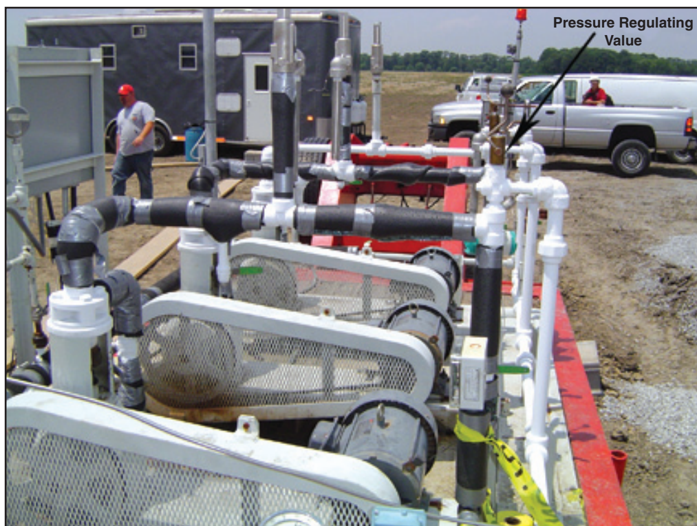
Figure 58. Pressure-regulating valves above and to the right of the Grainger motors (dark gray) above the frosted lines (see arrow, upper right). Photograph was taken by Ray McKaskle for Trimeric Corporation.
