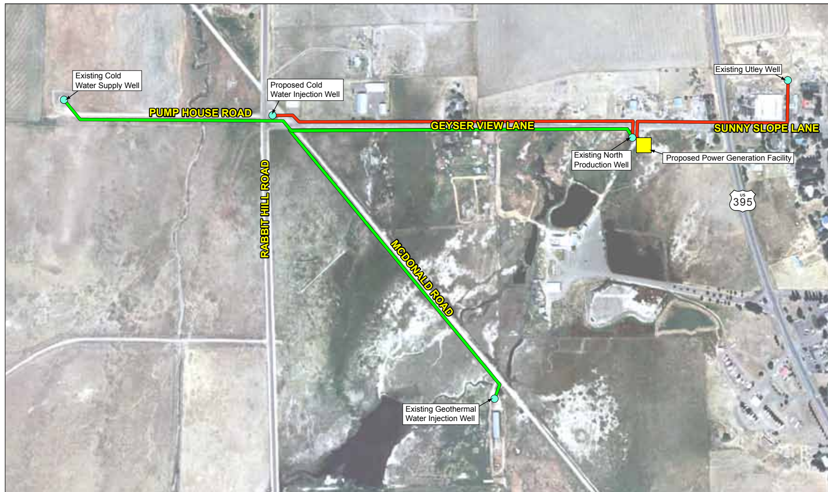
Figure 2: Location of Components of Geothermal Power Generation System
