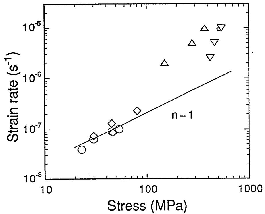
Figure 5. Creep results from five AlSiTi samples; each symbol represents a different sample.
