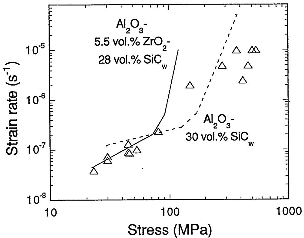
Figure 6. Creep data at 1400°C from this work (triangles) compared with creep of  $\text{Al}_2\text{O}_3$ -30 vol.% SiC whisker (dashed line) and  $\text{Al}_2\text{O}_3$ -5.5 vol.%  $\text{ZrO}_2$  particle-28 vol.% SiC whisker (solid line) composites.
