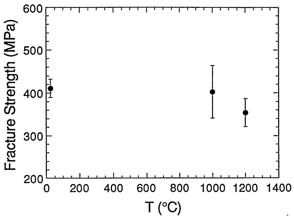
Figure 3. Four-point-bend fracture strength as a function of temperature.
