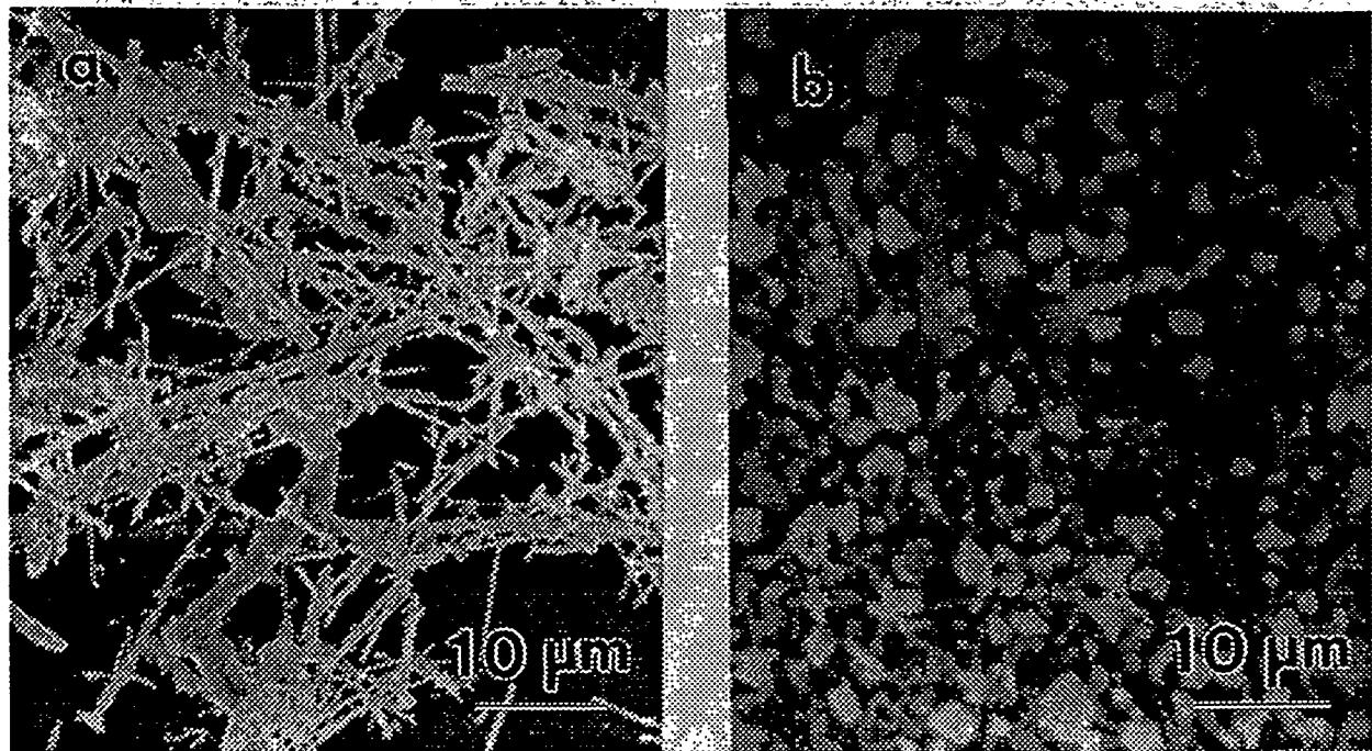
Figure 1. Optical photomicrographs of (a) SiC whiskers and (b) AlSiTi composite.
