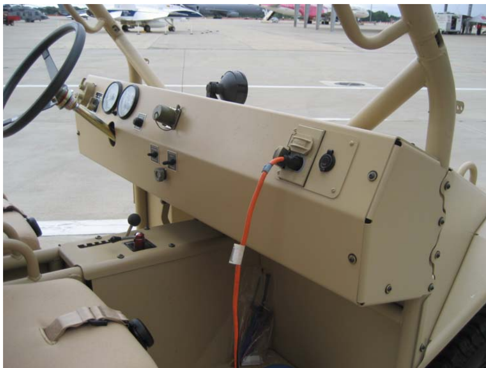
Figure 6: Auxiliary 115VAC outlet providing pure sine wave regulated electric power.
