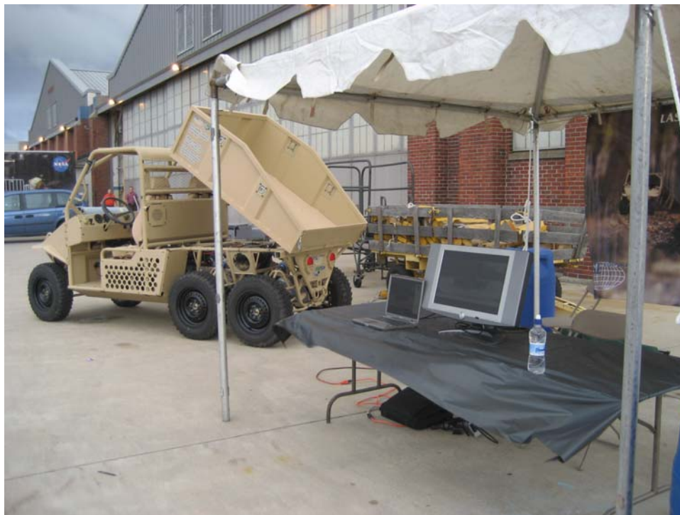
Figure 5: LASSO ® vehicle providing power to support laptop computer and LCD monitor.
