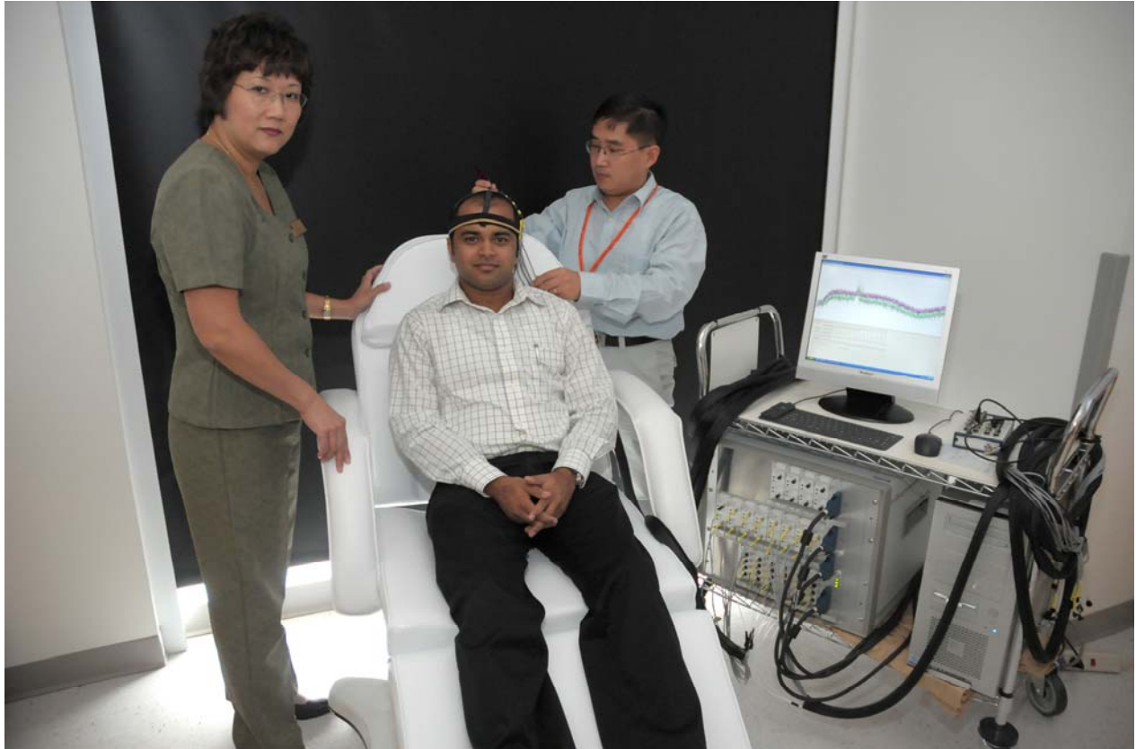
Figure 6: Dr. Hanli Liu, Professor of Bioengineering at UT Arlington and a co-principal investigator on this project (left), is demonstrating the multi-channel near infrared imager that she has acquired as part of this project and can be used to scan brain for brain blood flow oxygenation.
