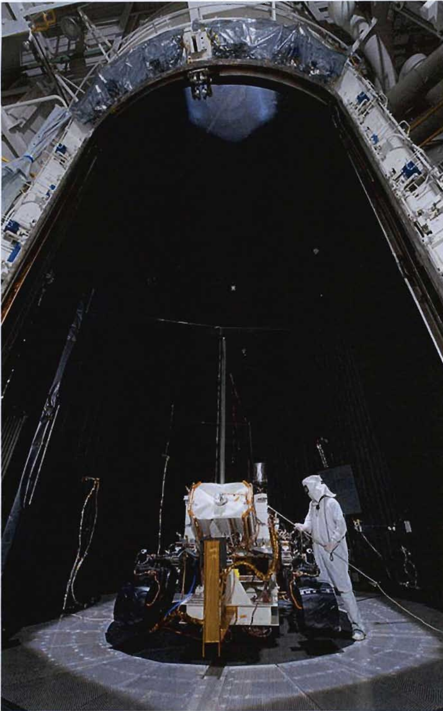
The Curiosity rover being prepared for the thermal environment test in March, 2011. Photo credit: JPL
