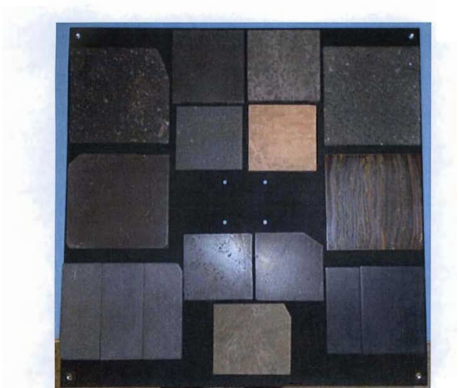
Rock slab targets for ChemCam arranged on a metal plate. This plate was positioned ~5 m (15 ft) from the rover during thermal testing. The panel measured about 2 feet (60 cm) square. Photo credit: JPL.
