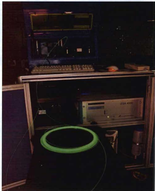
Figure4. In this picture is shown a general view of the Cart / Rack mounted LIBS system on the left and the system coupled to a 50 meter fiber optic cable illuminated with a green alignment laser for visual effects on the right hand side.
