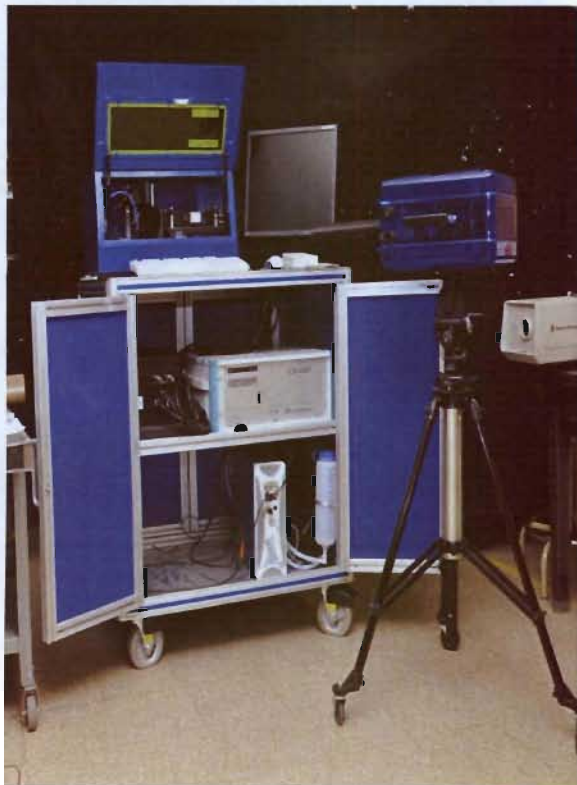
Figure4. In this picture is shown a general view of the Cart / Rack mounted LIBS system on the left and the system coupled to a 50 meter fiber optic cable illuminated with a green alignment laser for visual effects on the right hand side.
