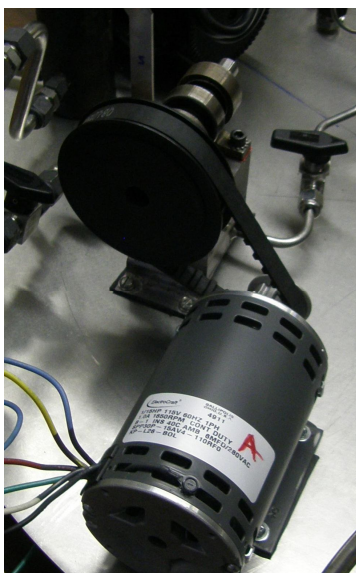
Figure 28: Solution Pump & Drive
