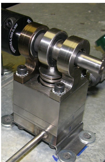
Figure 26: Prototype Solution Pump
