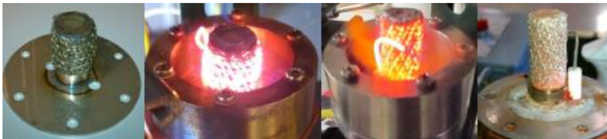
Figure 35: Radially-Fired Burners: SMTI "Short" (Left) and Solaronics (Right)
