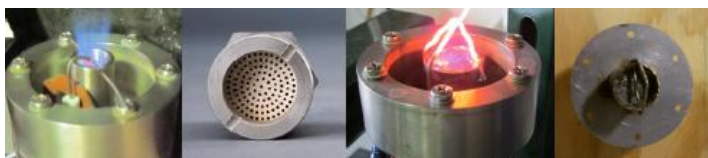
Figure 33: Selas Pilot Burner (Left); Micron-Fiber Burner (Right)
