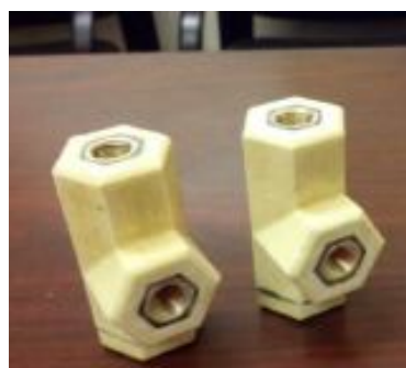
Figure 50: Rapid Prototype Fuel-Air Mixer
