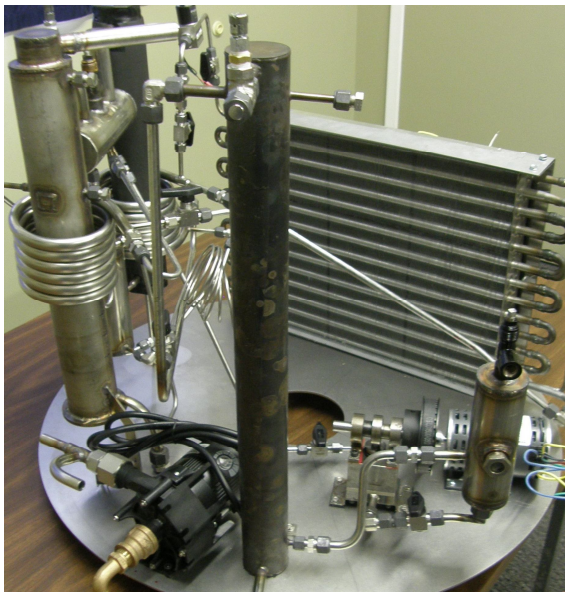
Figure 54: Alpha Prototype Heat Pump Sealed System
