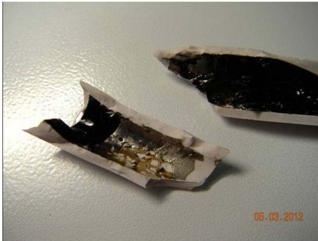
Figure 4.15. Secondary phase with metallic appearance observed on top of suction sample taken after Test 5 OX.
