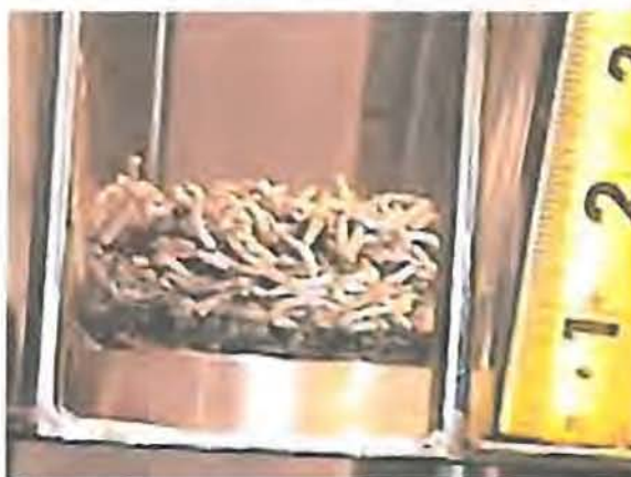
Fig.4: Aluminum Wire Observed in KOP Material.
