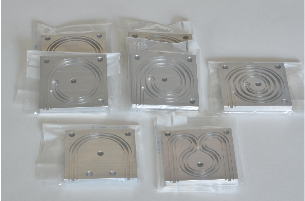
Figure 3. Meandering hollow waveguide prototypes were fabricated based on the design illustrations of Figure 1 using aluminum substrates with a final surface roughness of 100-200nm. The Fraunhofer IOF used the KERN Evo CNC Machine technology to fabricate these devices. A solid carbide end mill, HAM 430 precision milling tool (see Appendix E), was used for waveguide channel cuts. Note: the top plates for all waveguide devices were fabricated and polished at the Uni Ulm University Workshop.
