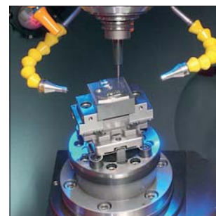
Ultra precision machining in hardened steel 47 HRC
