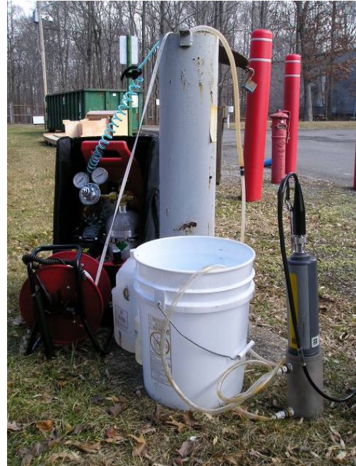
Exhibit 6-5. Well Monitoring Setup –Compressed Air, Water Depth. Meter, Discharge Collection Bucket, and Probe
