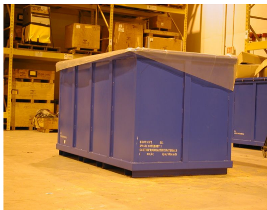
Exhibit 5-5. B-box with Liner in RWHF for Shipping Radioactive Waste to NTS
