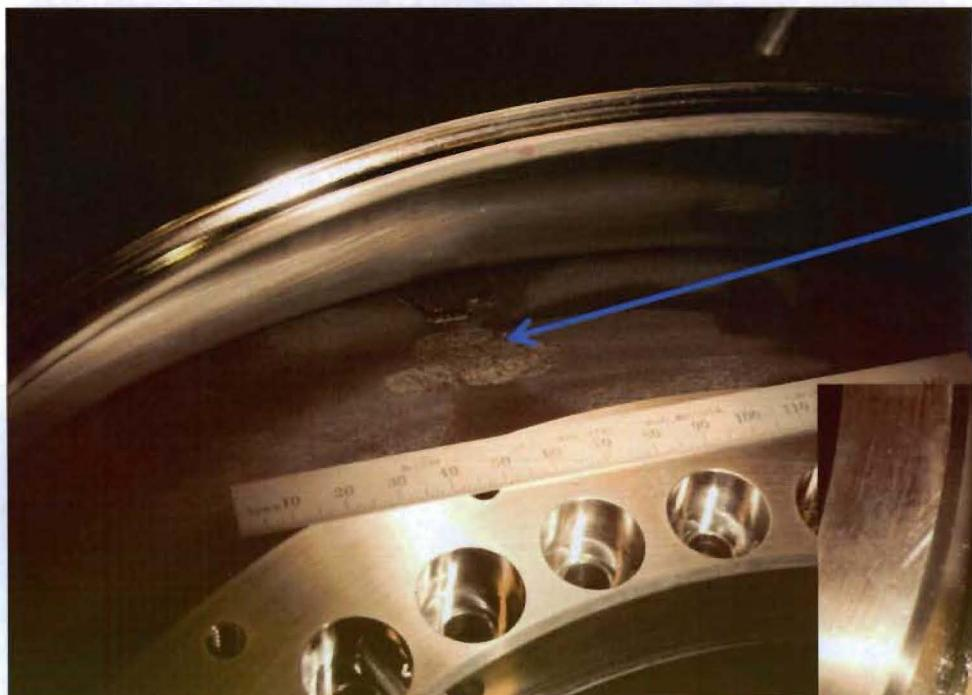
Spallation damage to one side of the insulator caused by the Arc
