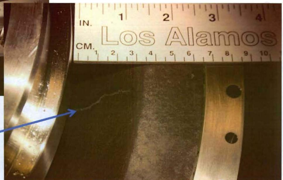
Arc damage to the other side of the insulator assembly
