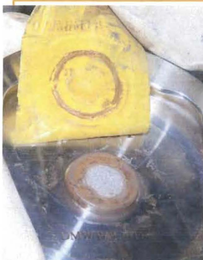
Filter region where tape was used at LANL to seal container before RH measurement, Residue was removed with tape
