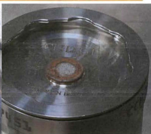
Filter region where tape was used at LANL to seal container before RH measurement, Residue was removed with tape
