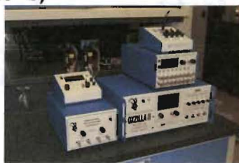
Ultrasensitive oxygen analyzer (Oxzilla II respirometer, Sable Systems)
