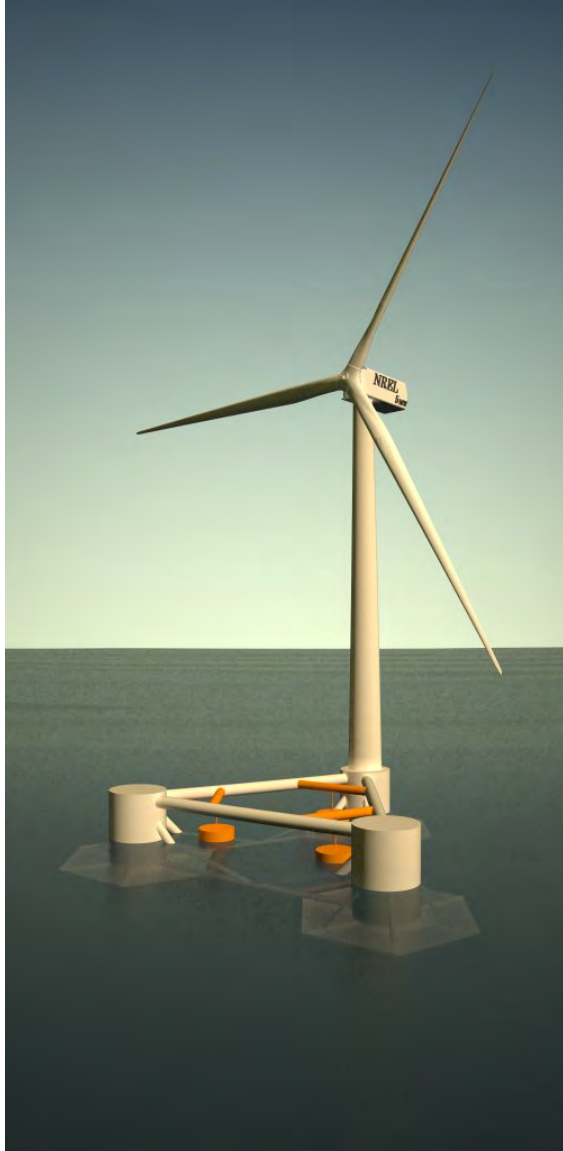
Figure 4: WindWaveFloat configuration 3, multiple point absorber.
