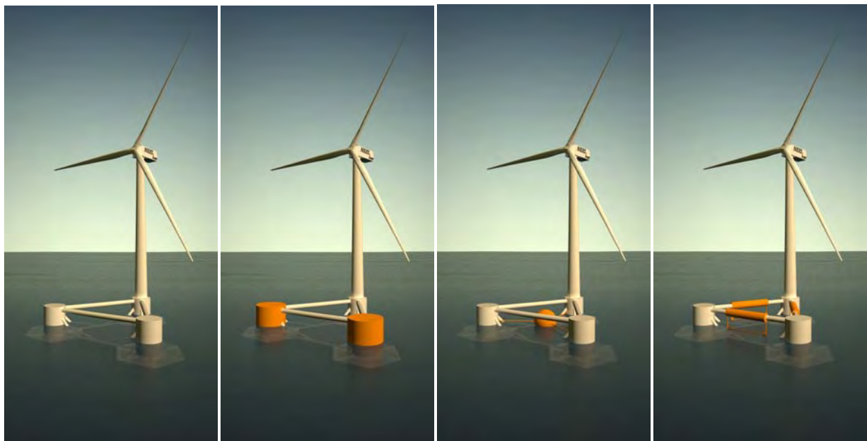
Figure 1: WindWaveFloat configurations (Base case, OWC, SWEDE, OWSC)
