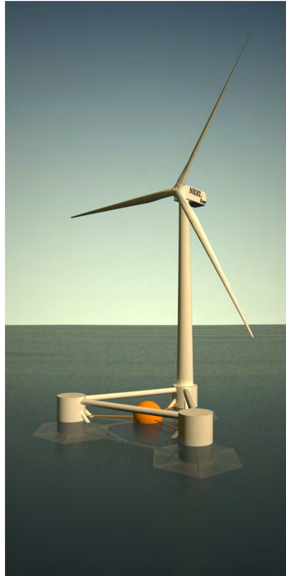
Figure 3: WindWaveFloat configuration 2, single point absorber (SWEDE)
