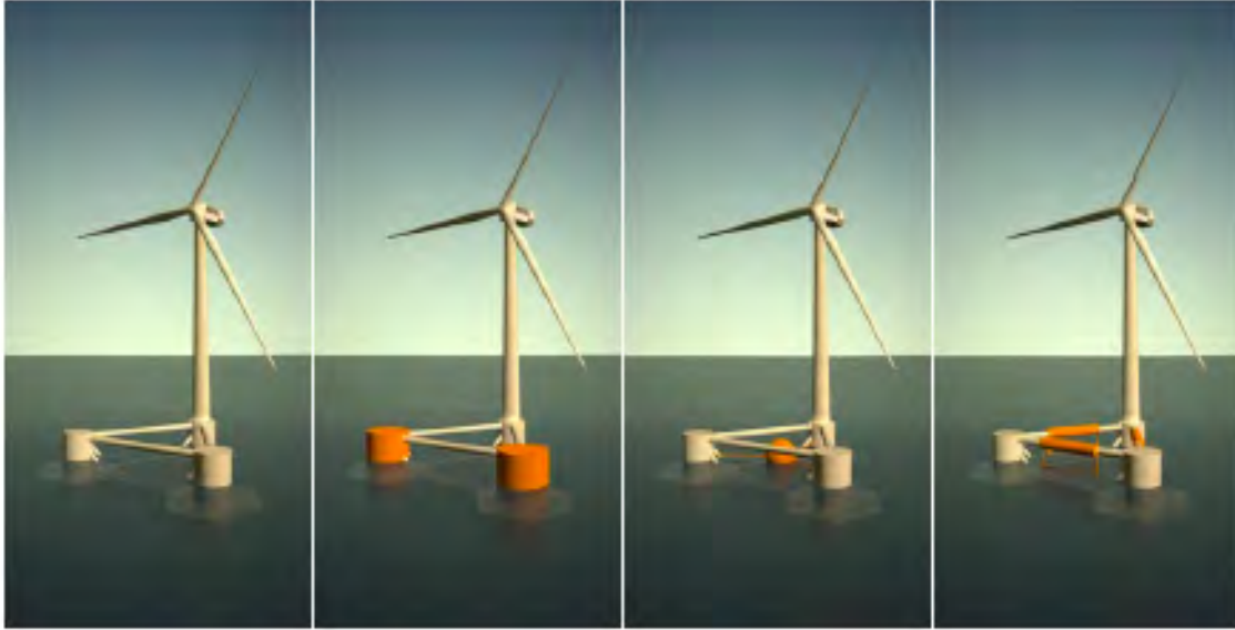
Figure 2: The base case WindFloat; oscillating water column, single point absorber and oscillating plates.
