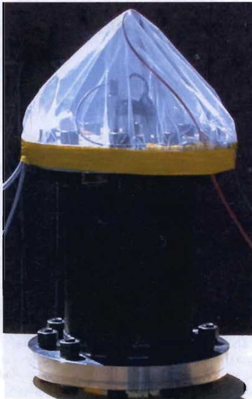
Figure 1 SECV assembly, top tent and cabling in place for testing
