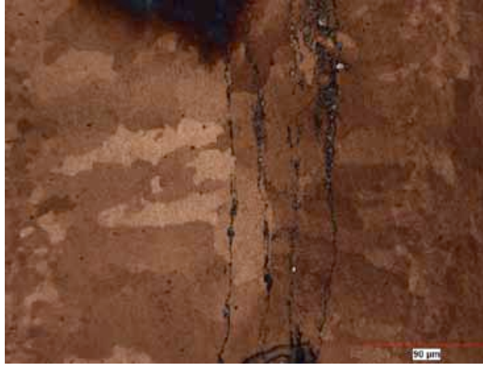
Figure 12: Optical image of spall plane in the HE driven as-annealed DU specimen. Note significant grain coarsening in the region of the spall plane, which runs vertically rather than horizontally in this image.
