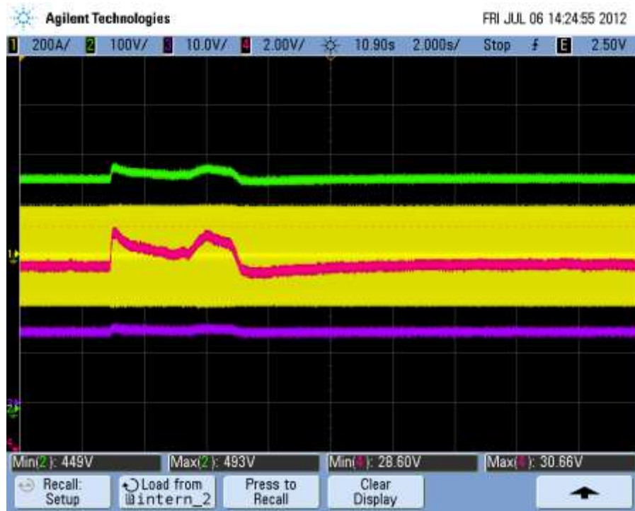
FIGURE 69: TRANSITION FROM 0 TO 25kW.
