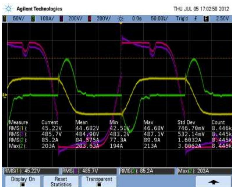
FIGURE 65: RESONANT WAVEFORMS FROM STEADY STATE TEST AT 50kW AVAILABLE AC POWER
