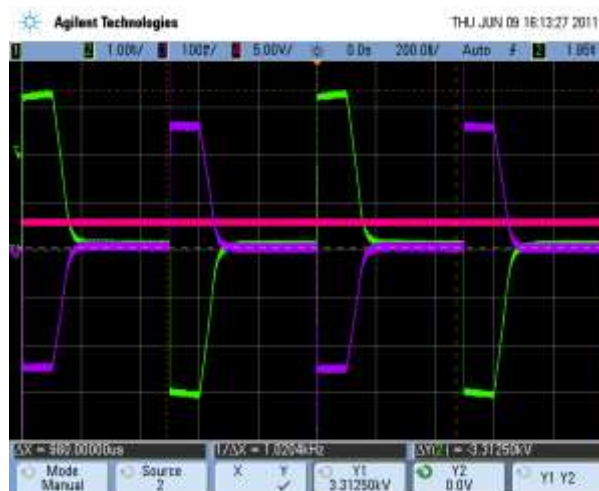
FIGURE 27: TEST DATA EXAMPLE SHOWING 3.312 kV, 1 kHz SWITCHING
