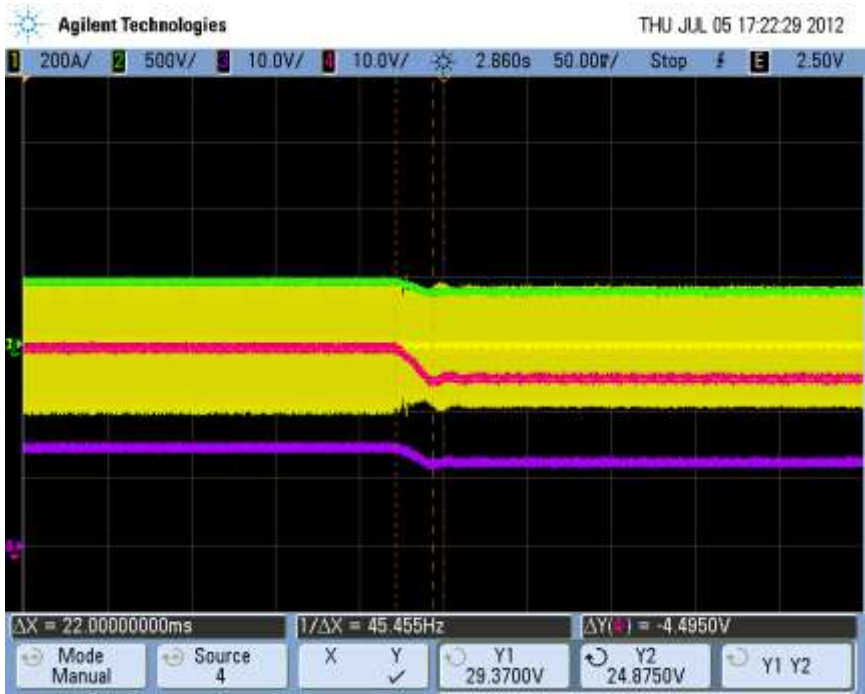
FIGURE 71: SUDDEN LOSS OF AC POWER.
