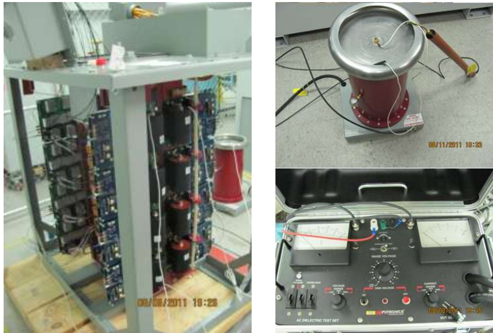
FIGURE 35: HI-POT TEST SETUP SHOWING TRANSFORMER (LEFT) AND HI-POT EQUIPMENT (RIGHT)
