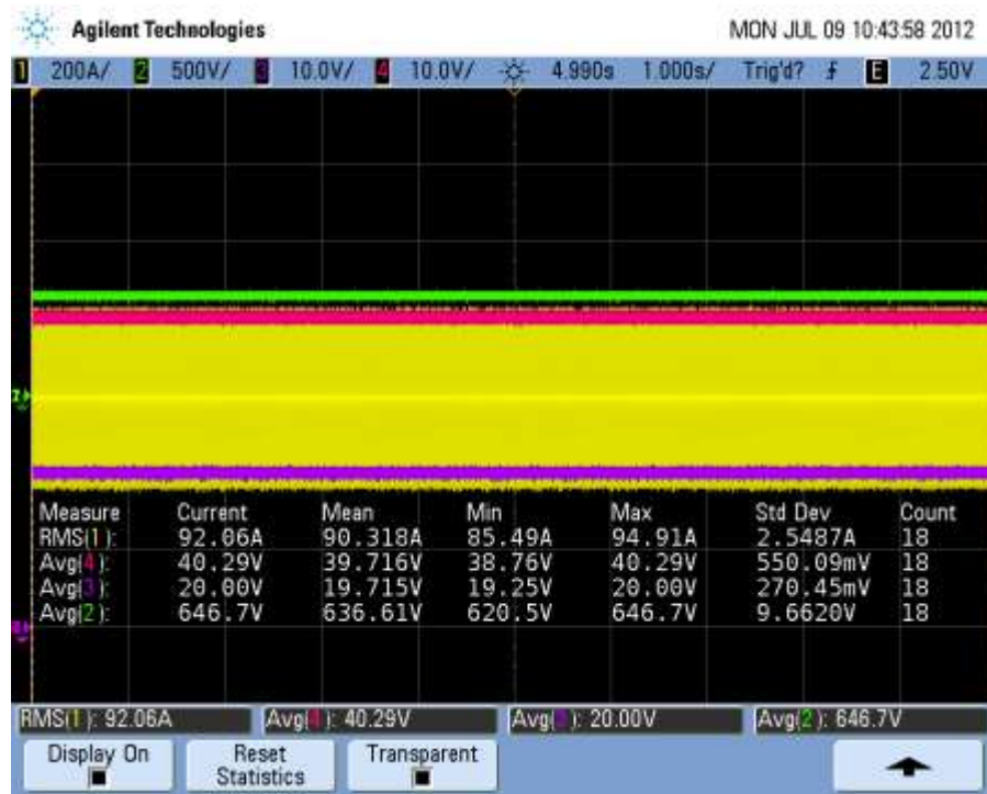
FIGURE 63: HIGHEST RECORDED OPERATION VOLTAGE OF 40.29kV (PINK, x1000), ACHIEVED USING 60US ON-TIME AND 70US DEAD TIME.
