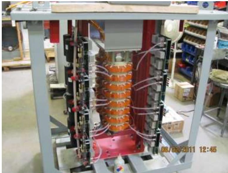
FIGURE 50: TRANSFORMER TEST FIXTURE BEFORE FINAL ASSEMBLY
