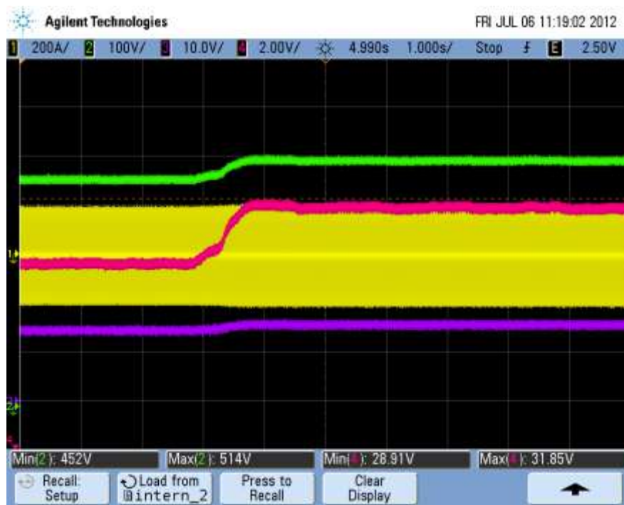
FIGURE 67:30kW TO 35kW AVAILABLE POWER TRANSITION.
