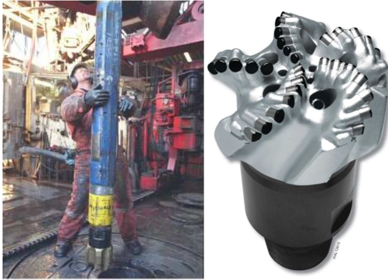
Figure 2-7. Diamond is used in drill bits and drilling tools and applied in the drilling of oil and gas wells. Shown are a steering assembly and a PDC drag bit.
