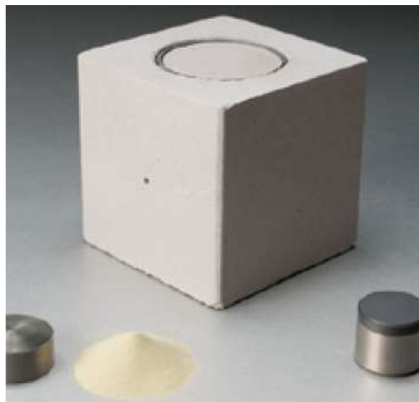
Figure 2-6. Diamond powder, tungsten carbide substrate (WC), high pressure/high temperature cube, and a complete diamond compact.
