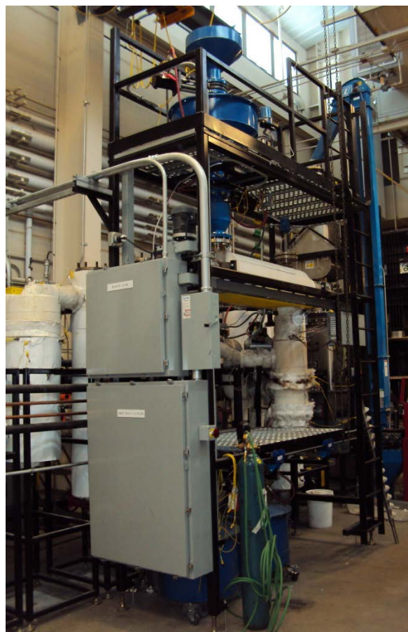
Figure 7: Moving Bed Granule Filter Process Development Unit
