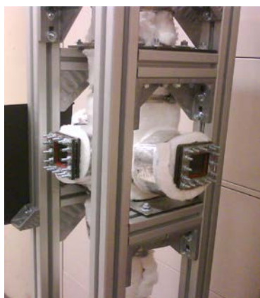
Fig. 4.11. Photograph of test section designed for insertion into pyrolysis production rig.
