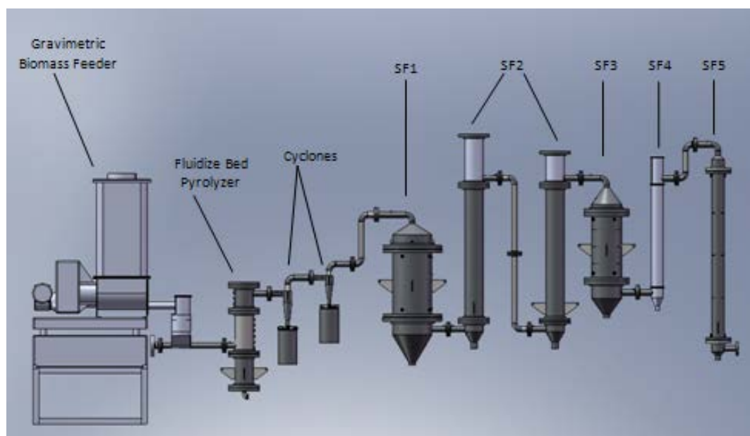
Figure 3.1. Process Development Unit (8 kg/hr) for stable bio-oil production
