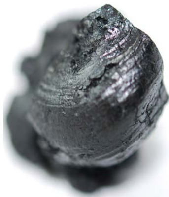
Figure 6: Char resulting from pyrolysis of red oak infused with 0.4wt% sulfuric acid.
