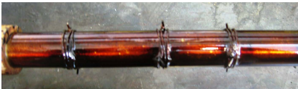
Figure 2. Modified ESP electrode after trial run
