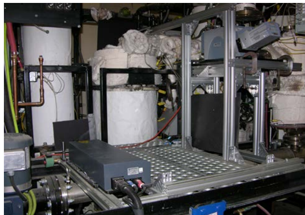
Fig. 4.12. Photograph of laser, optics, spectrometer, and camera installed in the pyrolysis oil pilot plant.
