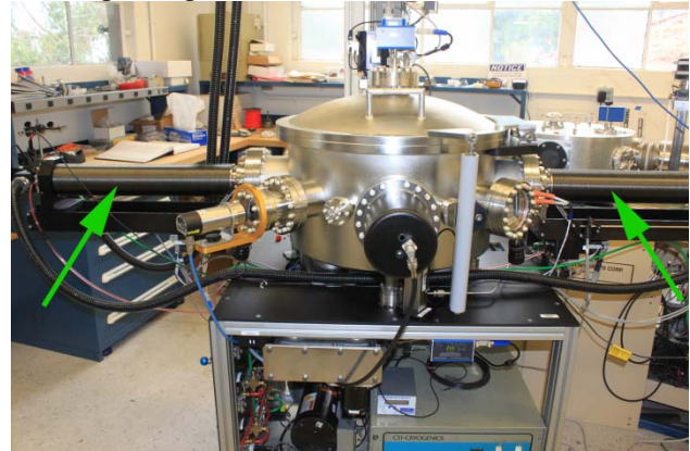
Figure 4: Deposition chamber dedicated to the coating of 1.3 GHz cavities with niobium using the HIPIMS process. The cylindrical magnetrons are mounted on opposing arms, indicated by the arrows, which allows them to slowly move in a synchronized manner driven by computer-controlled stepper motors.
