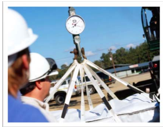
LiftPac bag lift test
