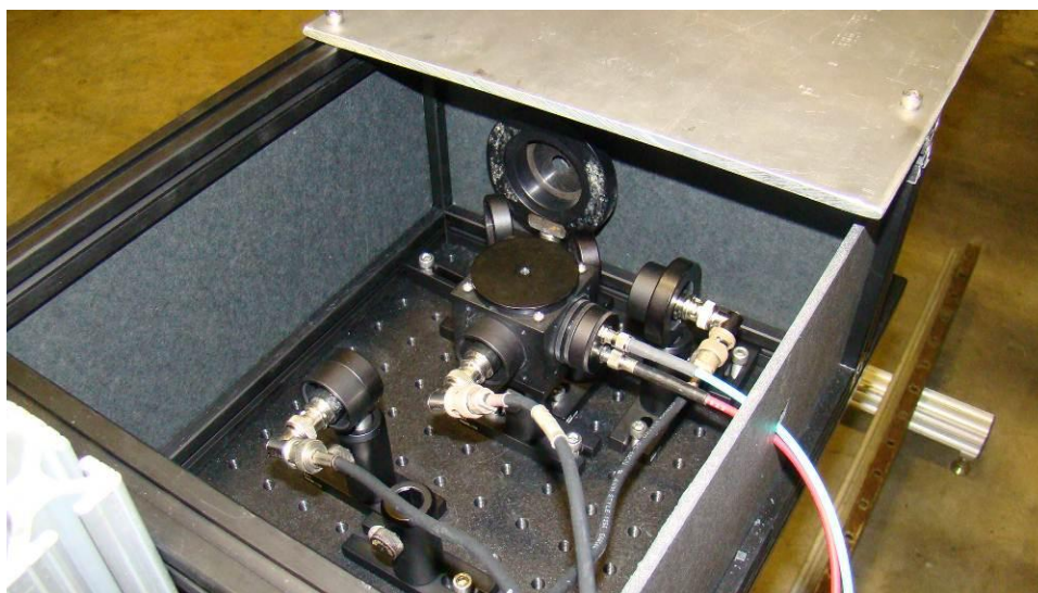
Figure 36. Intensity reduction apparatus for measuring spectrum of the plasma arc lamp.
