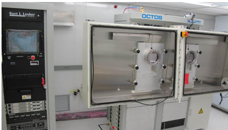
Figure 21. Dual-chamber (sputtering and thermal evaporation) system for CdTe research shown onsite in the 3500 clean room.
