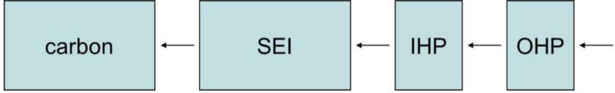
Figure 39: Schematic of COMSOL model regions and their interfaces.
