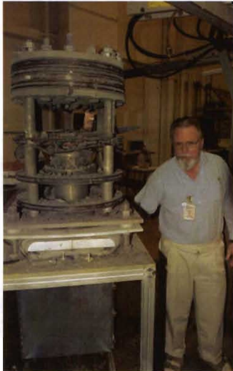
Project leader Jim Degan next to remains of the coils from the second engineering test shot.
