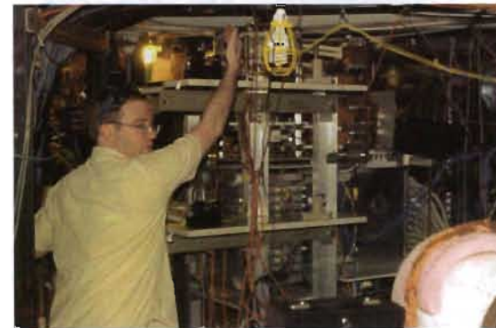
UNM scientist Alan Lynn adjusting 2-chord fiber interferometer on FRCHX
