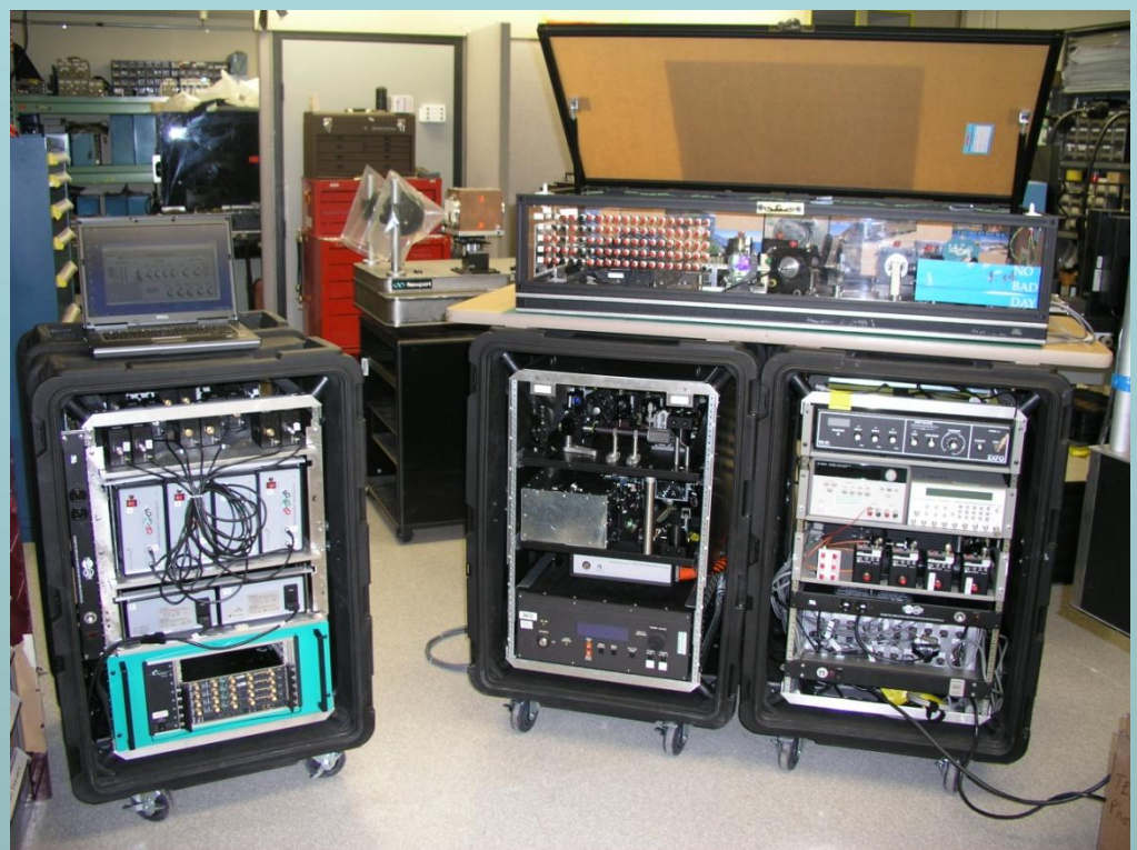
Fifteen channels of Fabry-Perot Velocimetry at NTS/U1a (circa 2003)
