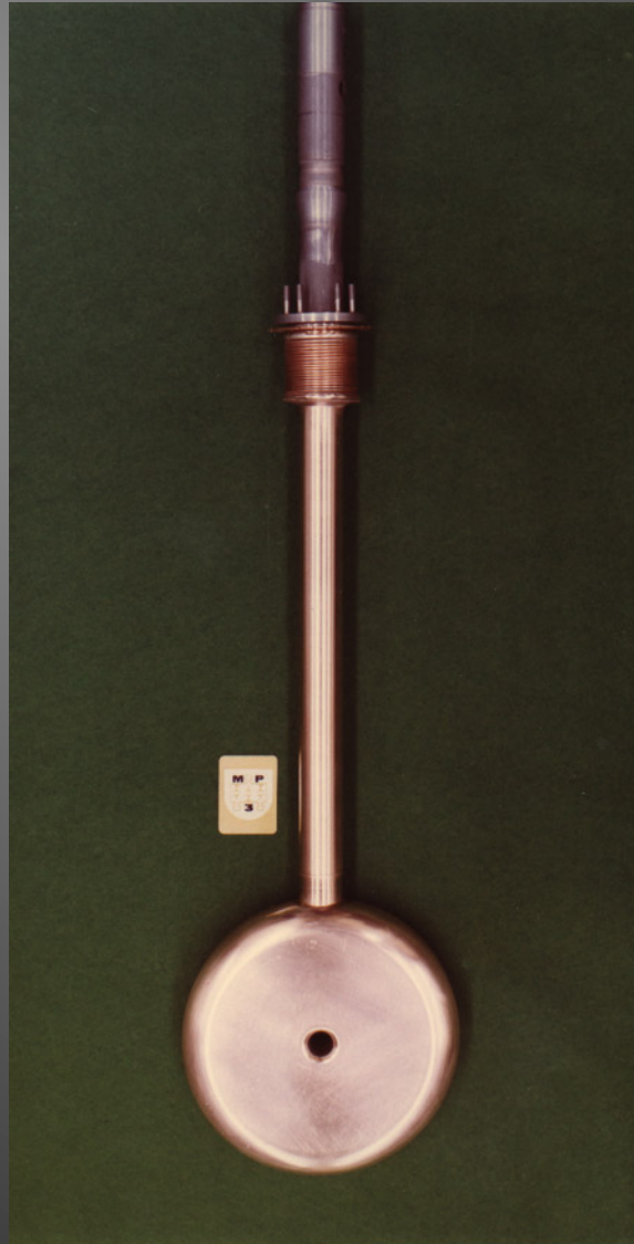
A low-energy drift tube fabricated by the group MP-3
