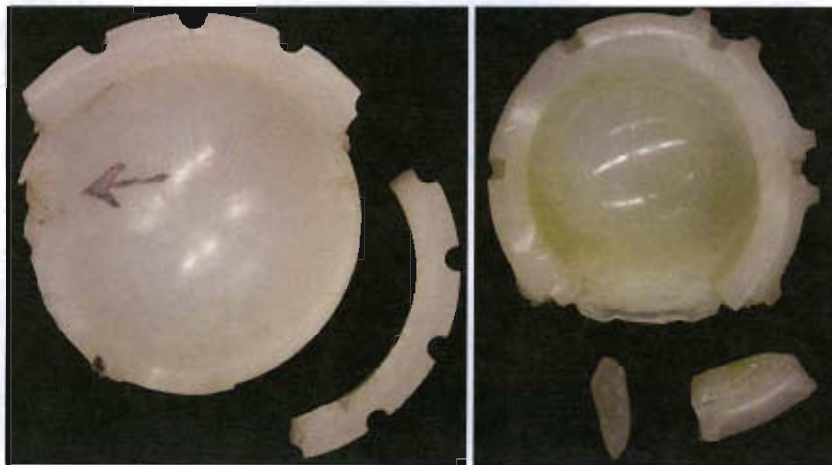
Fig.1 Two cross-linked UHMWPE total hip replacement bearings that fractured in patients under ordinary service conditions. Adapted from [4].
