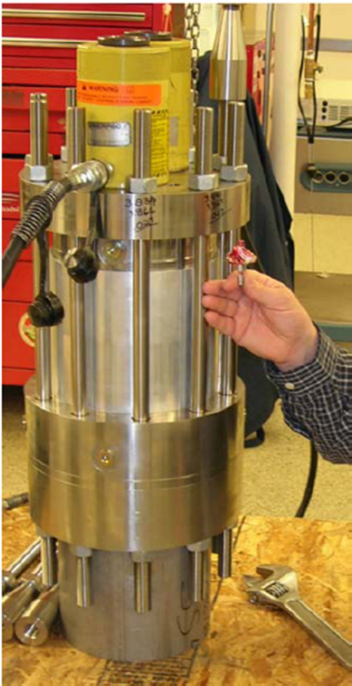
Figure 160 Supercritical carbon dioxide brayton cycle developed by Sandia National Laboratory and Barber-Nichols. (a) Assembled version of S-CO 2 cycle (b)
