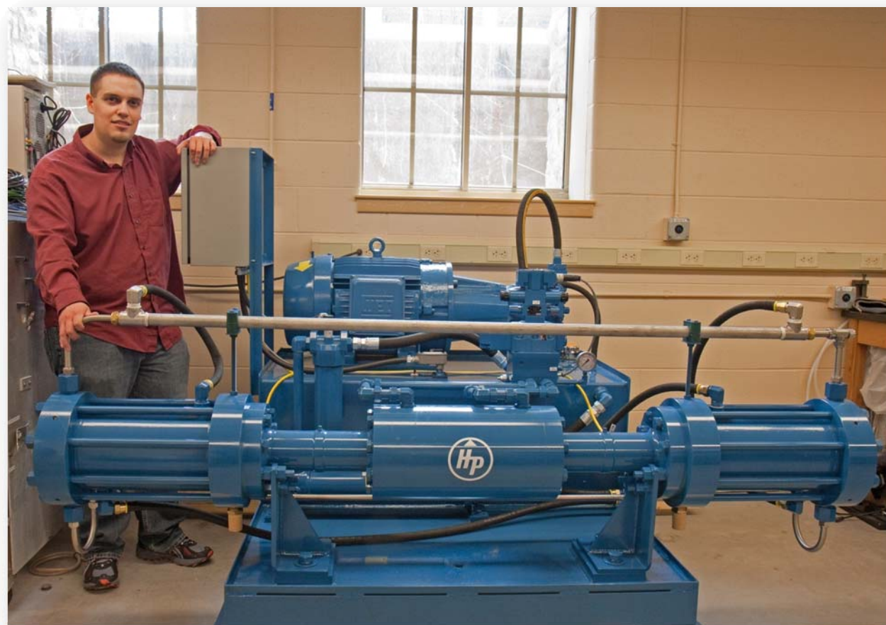
Figure 250 Hydro-Pac compressor to be installed Fall 2011
