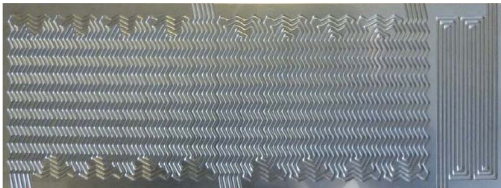
Figure 65: Image of a multi-stream PCHE plate from Le Pierres et al. [37].
