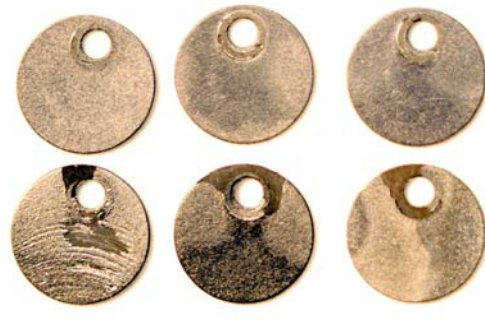
Figure 14 HCM12A samples after 500 hour exposure to s-CO 2 at 3000 psig
