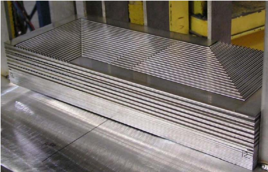
Figure 79: A photo of a hybrid PCHE and PFHE core, from Southall [40]. The channel perspective can make it difficult to identify, but from the top layer one can see a plate fin layer with side and end bars laid in the plain of the fin corrugations, a parting sheet, a printed circuit layer, and a total of 5 repetitions of this pattern.
