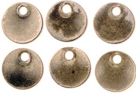
Figure 15 F91 samples after 500 hour exposure to s-CO 2 at 3000 psig
