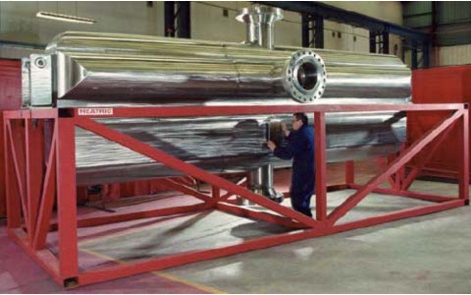
Figure 67: Image of a completed PCHE from Southall et al. [38].
