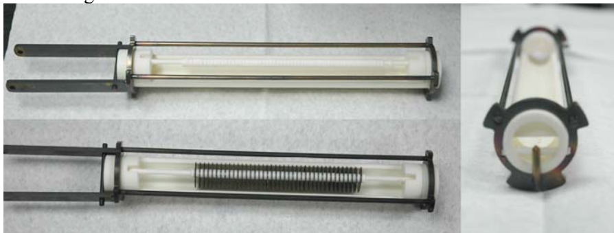
Figure 12 Sample boat in the inconel holder with the samples. The top photo shows the holes on the tabs used to lock the holder in place. Alumina washers separate the samples.
