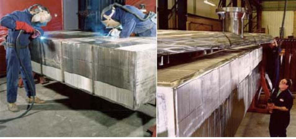
Figure 66: Images of welding and assembly of PCHE cores from Southall et al. [38].
