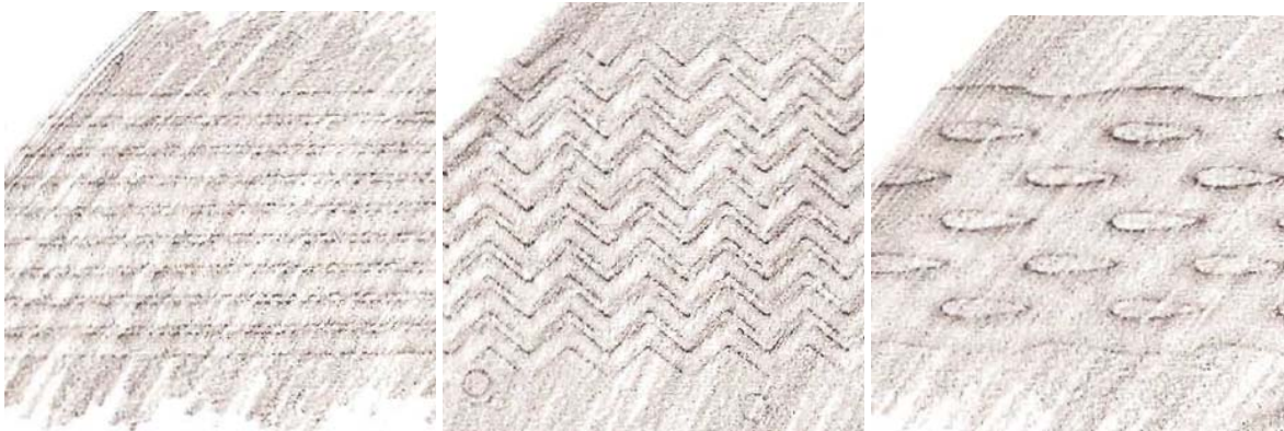
Figure 83: Example rubbings from 3 different PCHE plate surfaces (straight, zig-zag, and airfoil from left to right).
