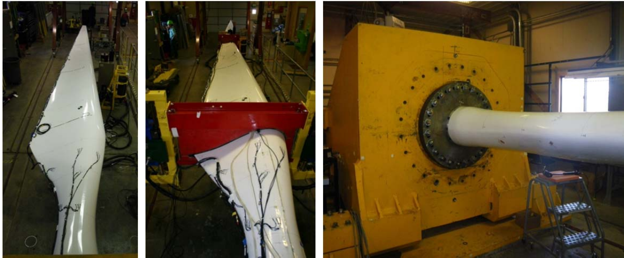
Figure 2. Fixed-free setup (left), mass-added setup (middle), and base fixture (right).
