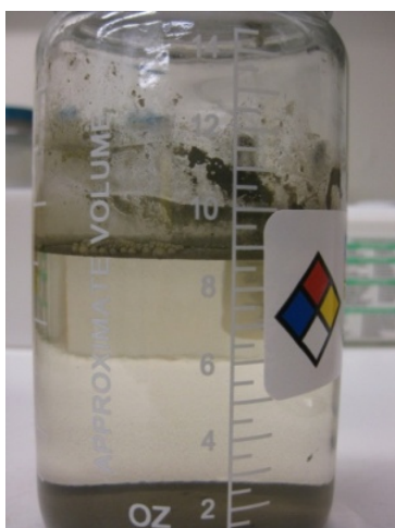
Figure 21: Reaction product liquor from wood reforming at 2% feed, 0.2 M \text{K}_2\text{CO}_3 , 310 °C, 0.6 L \text{min}^{-1} \text{N}_2 sweep gas and 7 g Raney Ni.
