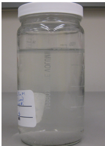
Figure 20: Reaction liquor from hydrolysis and liquid phase reforming of 5 wt% 100 mesh wood flour with Raney Ni and 0.2 M KOH at 310 °C.
