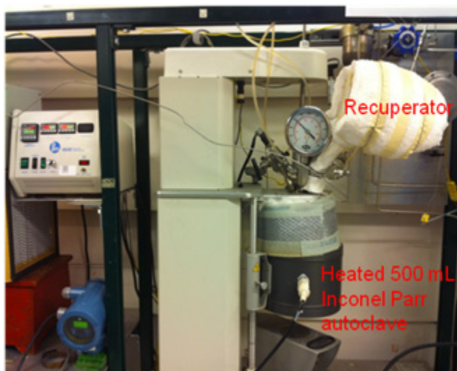
Figure 44: Continuous stirred tank reactor (CSTR) setup based on a 0.5 L Parr autoclave. Also shown is an insulated heat exchanger (recuperator) necessary to transfer heat from the CSTR effluent to the inlet for the autoclave heater to maintain a constant reaction temperature.
