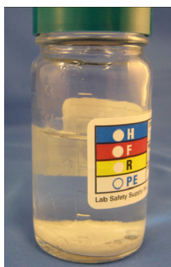
Figure 15: Reaction liquor obtained from the hydrolysis and Aqueous Phase Reforming of 1 wt% yellow poplar at 310 °C in 0.1M K 2 CO 3 , 0.5 slpm N 2 sweep gas, 1 g 2% Pt-1% Re/Ce 0.55 Zr 0.45 O 2 . (The white solid is potassium titanate.)
