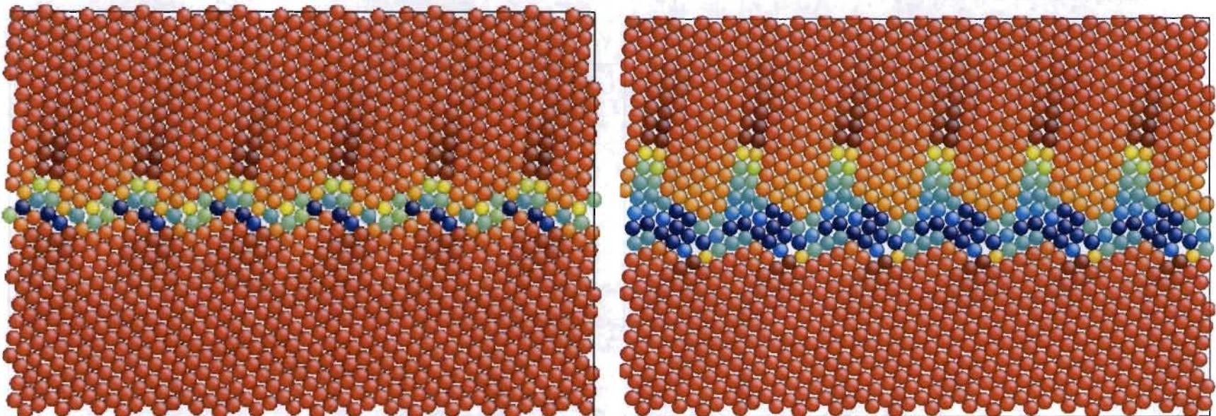
The atoms are colored by the order parameter where red color represent atoms in either of the two grains and blue color shows atoms that are disordered.
