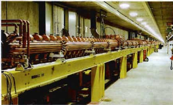
A Side-Coupled LINAC further increases the energy to 800 MeV
