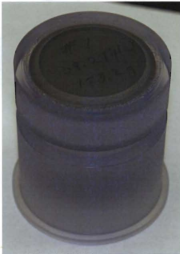
Projectile w. sample as impactor
